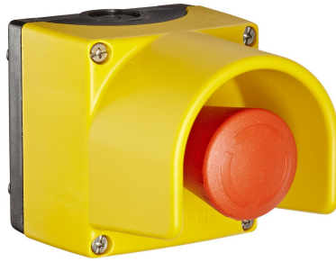
Figure 20. Emergency buttons are examples of an NC push-button switch. When the push button is released, the circuit is closed and current flows normally. However, when the push button is pressed (i.e., in the case of an emergency), the circuit becomes open and current ceases to flow in it (© Siemens AG 2014, all rights reserved).
