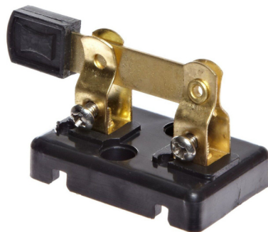
Figure 19. Example of a knife switch. The metal lever is currently inserted into the slot. Therefore, the switch allows current flow between its terminals.
