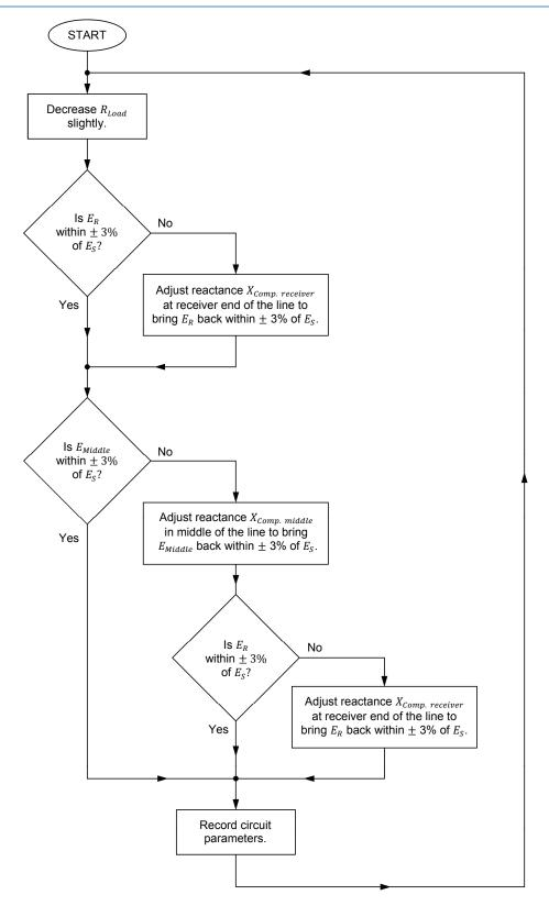
Figure 51. Algorithm used to control the distributed, switched shunt compensation.
