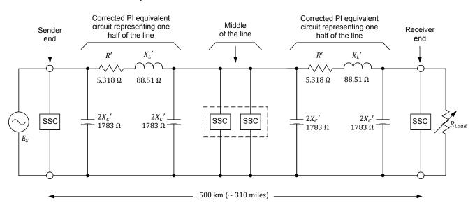
when it is voltage compensated using switched shunt compensation at both ends only.
