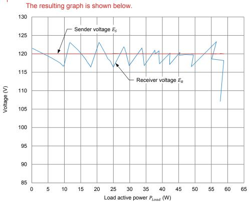
Power-voltage curve of the 700 km (about 435 miles) ac transmission line (for one phase) when distributed SSC (inductive and capacitive) is used for voltage compensation.
