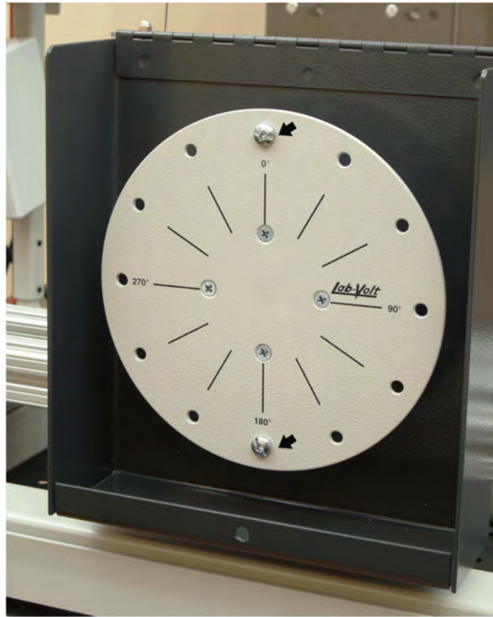
Figure 1-5. Balance the disk by installing a screw and a Keps nut.
