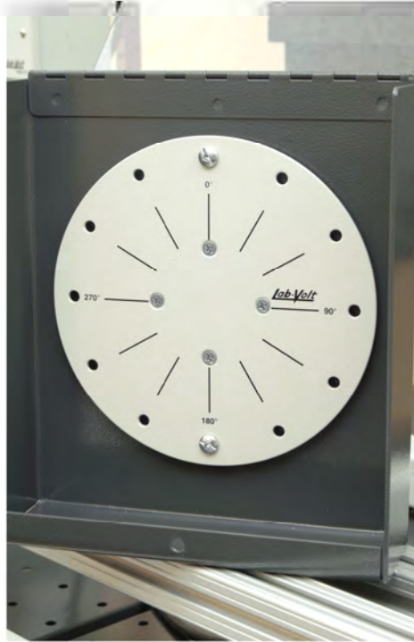
Figure 1-6. Storing the balancing disk in the cover.
