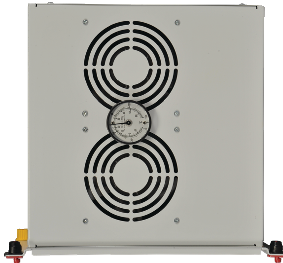
Figure 21. Radiator (rear view) with magnetic surface thermometer.
