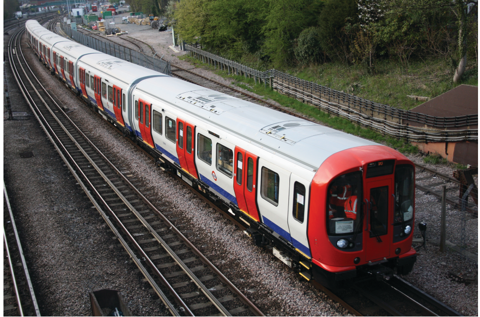
Figure 49. Certain London Underground public transportation trains are equipped with a regenerative braking system, allowing up to 20% of their input energy to be returned to the ac power network.
