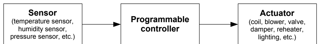
Figure 12. DDC controlled HVAC system operation.
