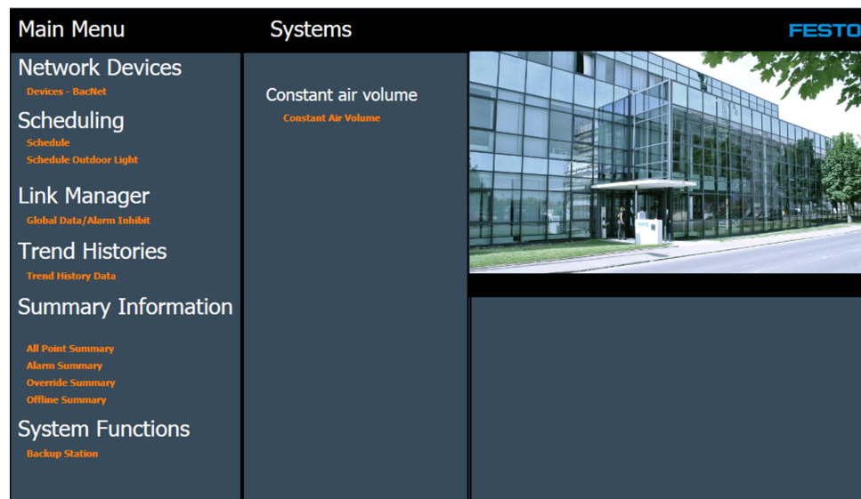
Figure 18. SCADA interface main window.
