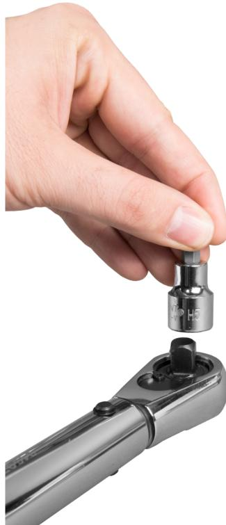
**Figure 17. Attach an H5 socket to the torque wrench.**
