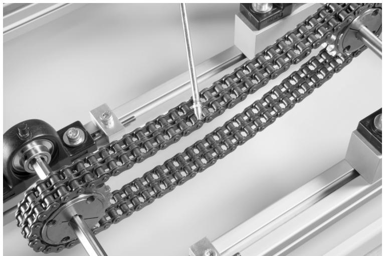
**Figure 27. Application of oil on the double-strand chain.**
