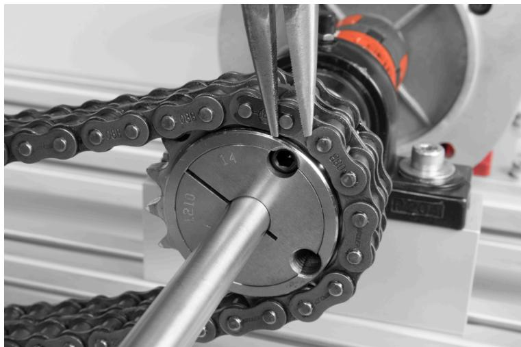
Figure 22. Locking clip installation.
