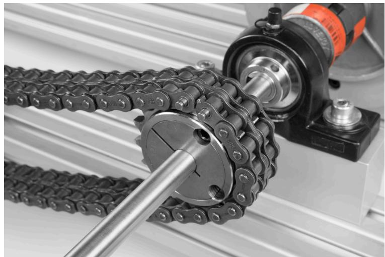
Figure 20. Pushing the plate with pins through the ends of the double-strand chain.
