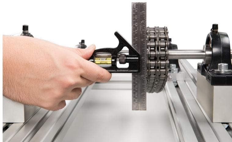
**Figure 24. Vertical angular alignment.**
