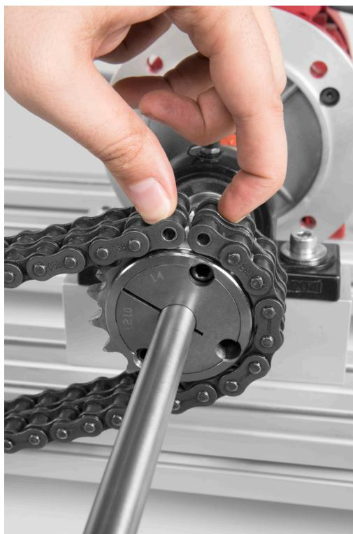
Figure 18. Lay the double-strand roller chain on the sprockets.
