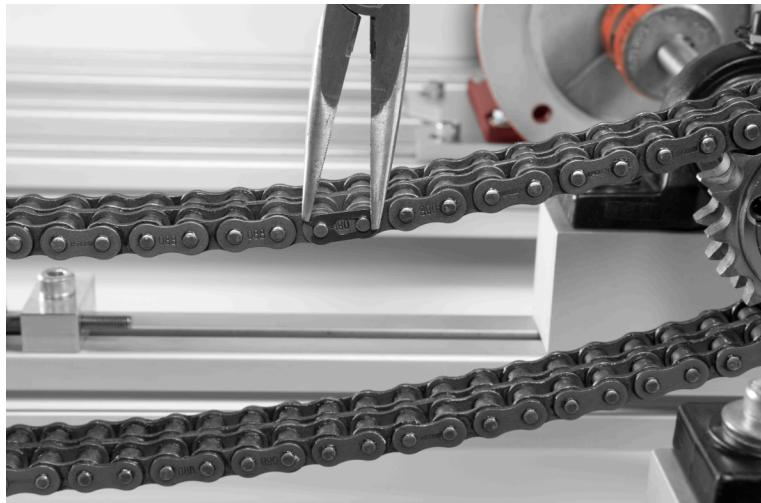
Figure 28. Connecting link dismantlement.
