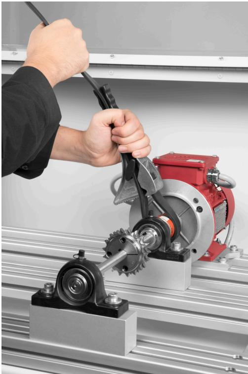
**Figure 16. Grip the jaw coupling using the strap wrench.**
