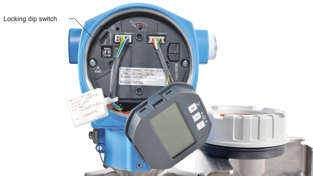
Figure 2-11. Position of the locking dip switch.
