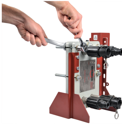
Figure 2-12. Loosening the compression bolts.
