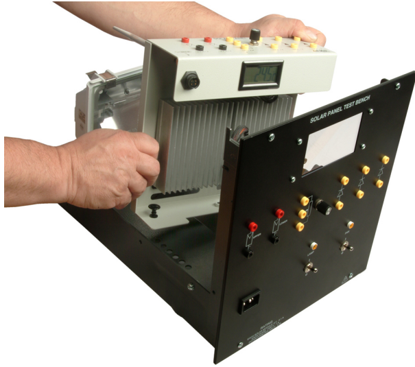
Figure 32. Installing a solar panel in the Solar Panel Test Bench.
