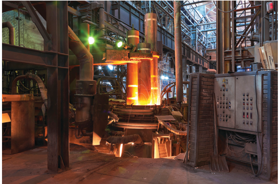
Figure 91. SVCs can be used near electric arc furnaces to reduce the voltage fluctuations caused by the flicker (sudden and erratic variations in the length of the furnace arc).
