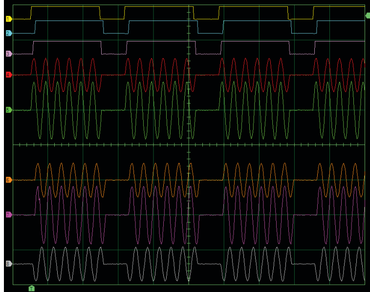
Firing signals of thyristors Q_1 , Q_2 , and Q_3 and waveforms of load currents and voltages (duty cycle \alpha set to 75%).
