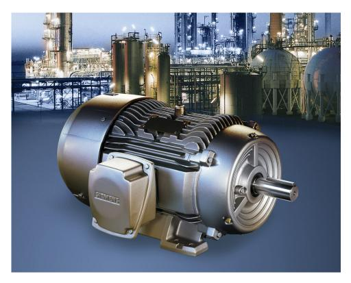
Figure 2-8. Three-phase induction motors are the most commonly used alternating current motors in industrial applications worldwide. This is primarily due to the fact that induction motors are simple, robust, and relatively cheap compared to other types of alternating current motors (© Siemens AG 2012, all rights reserved).
