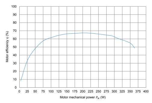
Three-phase induction motor efficiency  $\eta$  as a function of the motor mechanical power  $P_M$ .
