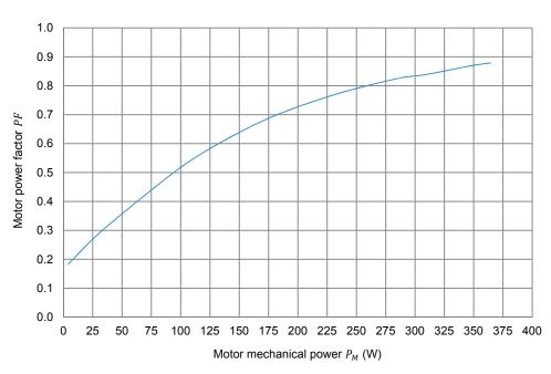
Three-phase induction motor power factor PF as a function of the motor mechanical power  $P_{M}$ .
