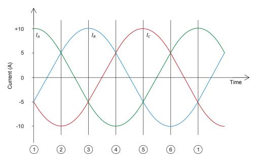
Figure 2-6. Three-phase sine wave currents flowing in the stator windings.
