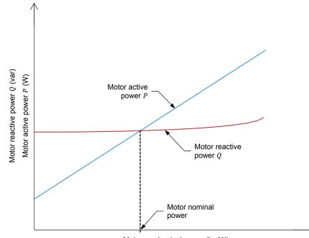
Motor mechanical power  $P_M$  (W)
