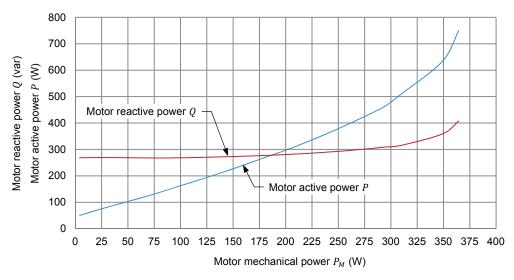
Three-phase induction motor active power P and reactive power Q as a function of the motor mechanical power  $P_M$ .
