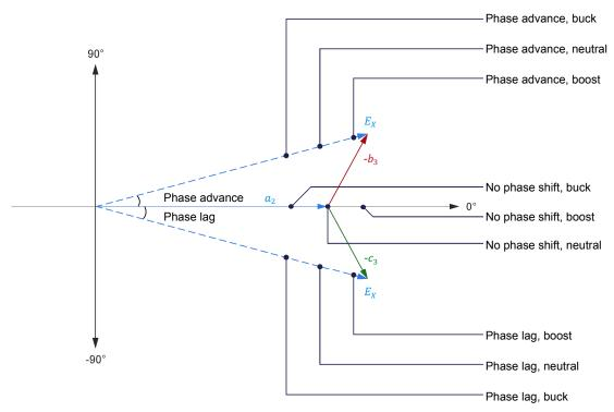
Figure 41. Phasor diagram of the outgoing voltages possible at one phase of a regulating autotransformer acting as both a phase-shifting transformer and a buck-boost transformer.
