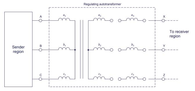
Figure 38. Equivalent circuit of a regulating autotransformer.
