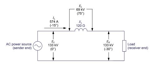
Figure 32. Voltage-compensated 230 kV ac transmission line.
