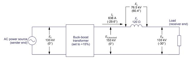
Figure 34. Voltage-compensated 230 kV ac transmission line of Figure 32 with a buck-boost transformer added at the sender end of the line.
