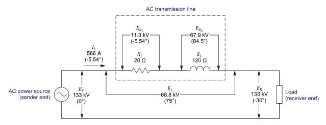
Figure 36. Voltage-compensated 230 kV ac transmission line of Figure 32 when the line resistance  $R_L$  is assumed to be equal to 20  $\Omega$ .
