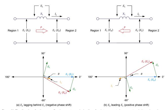
Figure 29. The direction of active power flow in an ac transmission line of an interconnected power network depends on the polarity of the phase shift  $\theta$  between the voltages at both ends of the line.
