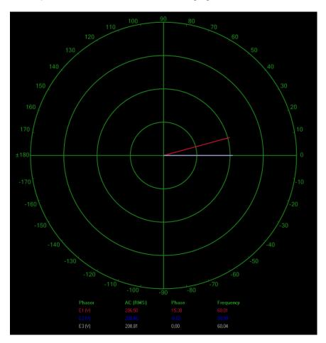
Phasors of the voltage  $E_{Reg,A}$  at region A, the modified voltage  $E'_{Reg,A}$  at region A, and the voltage  $E_{Reg,B}$  at region B when the Regulating Autotransformer is set to a +15° phase shift.
