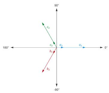
(b) Phasor diagram of the voltages at the secondary and tertiary windings
