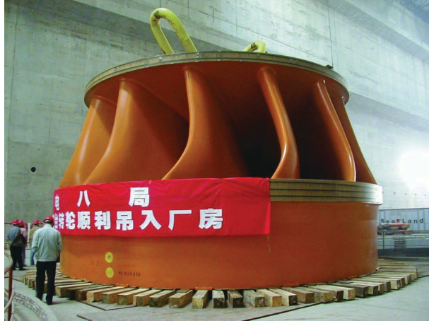
Figure 11. One of the 29 currently installed Francis turbines in the Three-Gorges Dam hydropower plant in China. Each turbine has a power generating capacity of 700 MW (photo courtesy of Voith Siemens Hydro Power Generation).
