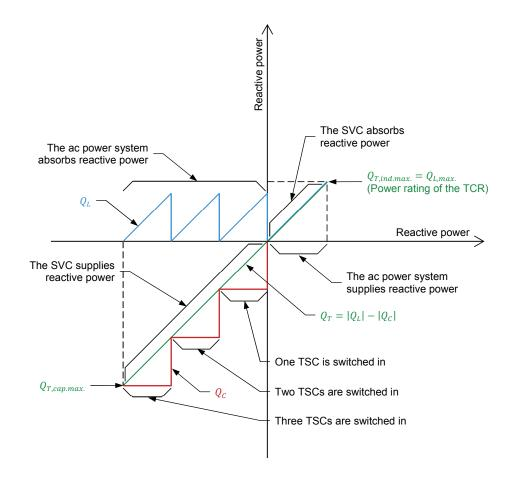
Figure 36. Reactive power exchange characteristic of an SVC of the TCR-TSC-type.
