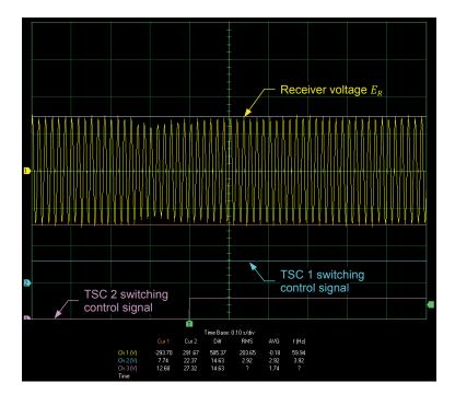
Receiver voltage  $E_R$ , TSC 1 switching control signal, and TSC 2 switching control signal when the SVC compensates the voltage at the receiver end of an ac transmission line and the load increases.
