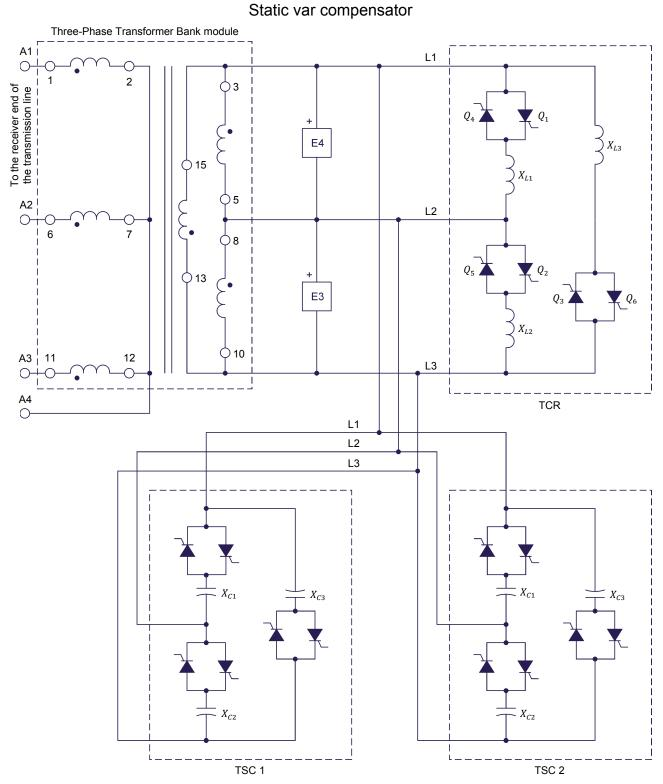
Figure 43. Circuit for studying the operation of an SVC used for voltage compensation of an ac transmission line supplying power to a resistive load.
