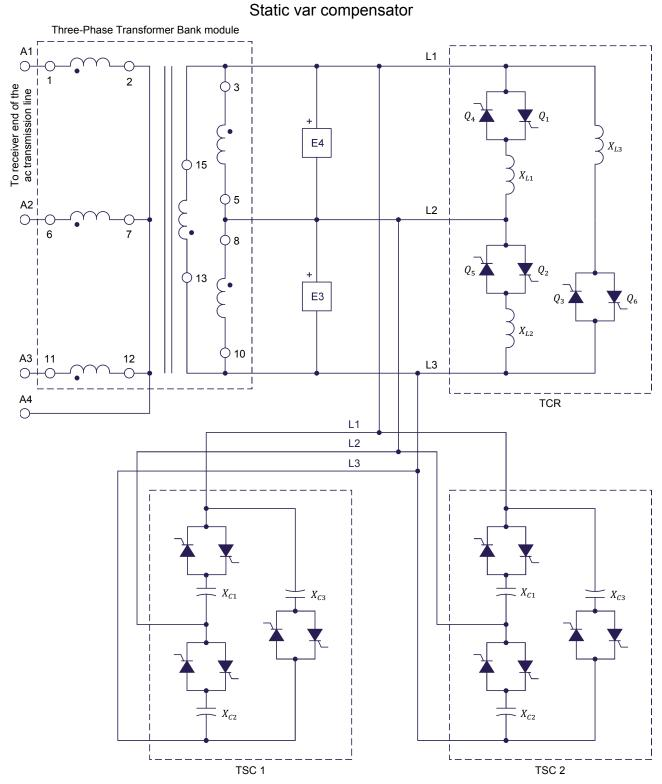
Figure 45. Circuit for studying the operation of an SVC used for voltage compensation of an ac transmission line containing a shunt-capacitor substation.
