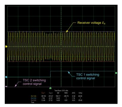
Receiver voltage  $E_R$ , TSC 1 switching control signal, and TSC 2 switching control signal when the SVC compensates the voltage at the receiver end of a long ac transmission line and the voltage compensation provided by the shunt-capacitor substation decreases.
