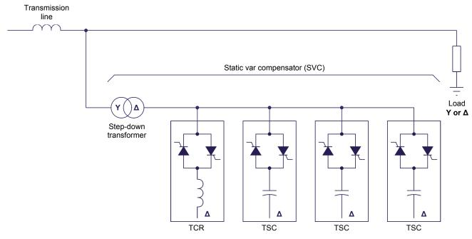
Figure 34. Simplified single-wire circuit diagram of an SVC of the TCR-TSC type.
