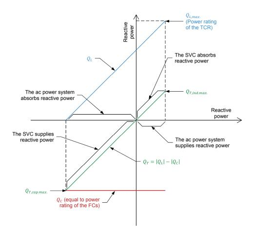
Figure 33. Reactive power exchange characteristic of an SVC of the TCR-FC-type.
