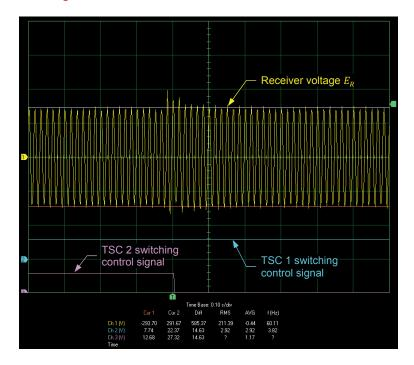
Receiver voltage  $E_{R}$ , TSC 1 switching control signal, and TSC 2 switching control signal when the SVC compensates the voltage at the receiver end of an ac transmission line and the load decreases.
