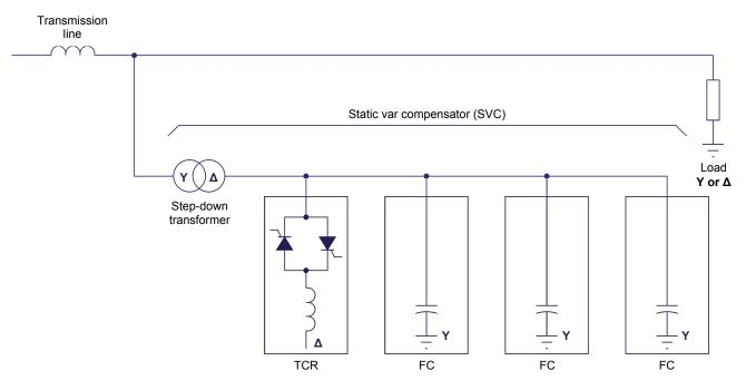
Figure 31. Simplified single-wire circuit diagram of an SVC of the TCR-FC type.
