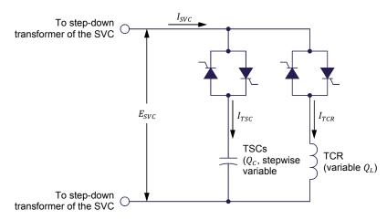
Figure 35. Simplified circuit diagram of one leg (phase) of an SVC of the TCR-TSC type showing the main voltage, current, and reactive power parameters.
