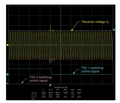
Receiver voltage  $E_R$ , TSC 1 switching control signal, and TSC 2 switching control signal when the SVC compensates the voltage at the receiver end of a long ac transmission line and the load decreases.
