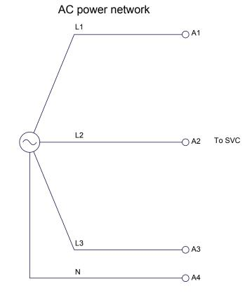
Figure 40. Circuit for measuring the reactive power capacity of an SVC consisting of one TCR and two TSCs.
