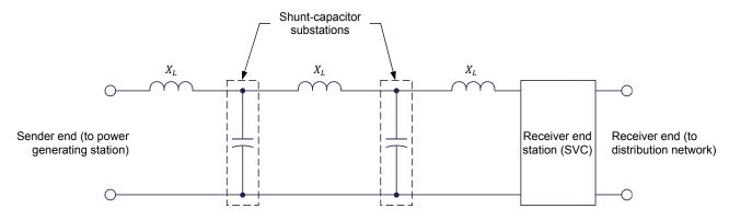
Figure 29. Typical ac transmission line used to transfer large amounts of electrical power over a long distance from a power generating station to the distribution network.
