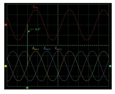
Sine waves of the line voltages at the primary and the secondary of the three-phase transformer bank when it is connected in a delta-delta configuration.
