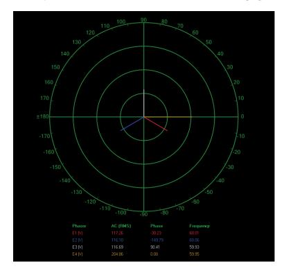
Phasors of the line voltages at the primary and the secondary of the three-phase transformer bank when it is connected in a wye-delta configuration.
