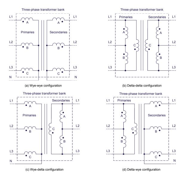
Figure 3. The four most common three-phase transformer configurations.
