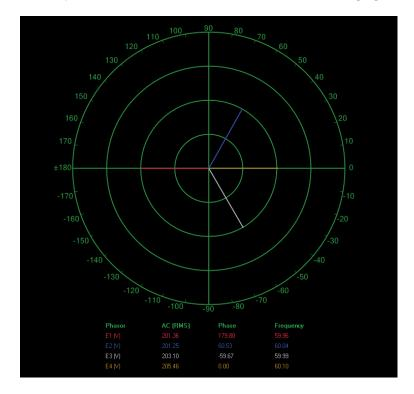
Phasors of the line voltages at the primary and the secondary of the three-phase transformer bank when it is connected in a delta-delta configuration with reversed connections at the secondary windings.
