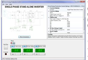
The Home Energy Production Control Function Set enables the following devices required for home energy production to be implemented using the Data Acquisition and Control Interface, the IGBT Chopper/Inverter, and the Insulated DCto-DC Converter:
