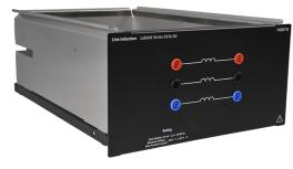
The Line Inductors module consists of three separate inductors enclosed in a half-size EMS module to be connected in series in a three-phase circuit. Six safety banana jacks provide individual access to each inductor. The Line Inductors are used to limit the rate of change of line currents in three-phase ac power systems.
