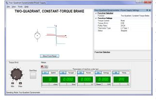
The Standard Functions (computer-based control) Set is a package of control functions that can be activated in the Four-Quadrant Dynamometer/Power Supply, enabling the module to perform a wide variety of functions in each of its two operating modes (Dynamometer and Power Supply).
