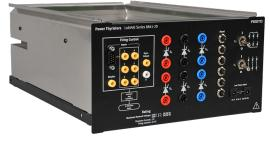
The Power Thyristors module consists of six power thyristors (SCRs) mounted in a half-size EMS enclosure. Each individual thyristor is protected against overcurrents and short-circuits. All the anodes and cathodes of the thyristors are terminated on the front panel by color-coded, 4 mm safety banana jacks. To reduce the number of external connections, the most typical thyristor configurations can be achieved through the use of two toggle switches on the front panel.
