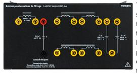
This Filtering Inductors/Capacitors module consists of two separate filters enclosed in a half-size EMS module: a lowfrequency filter and a high-frequency filter. The low-frequency filter consists of an inductor and a polarized capacitor, while the high-frequency filter consists of two inductors and a nonpolarized capacitor. Internal electrical components are identified on the module front panel. 4 mm banana jacks provide access to the different components in the module.
