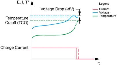
This function uses the four-quadrant power supply to implement an advanced Ni-MH battery charger. This charger forces a constant charge current in the battery until the battery voltage, which increases steadily from the beginning of charge, reaches a plateau and decreases by a certain amount (-dV), at which point the charge terminates. The charger also monitors the battery temperature during charge. Battery charging is terminated immediately when the
