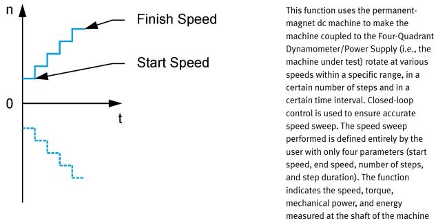
under test. The function can also indicate the machine temperature when the temperature sensor of the machine under test (if so equipped) is connected to the Thermistor Input of the Four-Quadrant Dynamometer/ Power Supply. The Speed Sweep function is useful to measure how parameters related to the machine under test vary as a function of the rotation speed. The parameters measured throughout the speed sweep can be recorded to a data table automatically.
