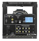
The Four-Quadrant Dynamometer/ Power Supply mainly consists of a permanent-magnet dc motor, a fourquadrant power supply, and an onboard microcontroller enclosed in a full-size EMS module. A toggle switch on the front panel allows selection of the operating mode (Dynamometer or
