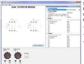
The High-Voltage DC (HVDC) Transmission System Control Function Set enables the following devices required for the study of HVDCs to be implemented using two Data Acquisition and Control Interface, and two Power Thyristors:
