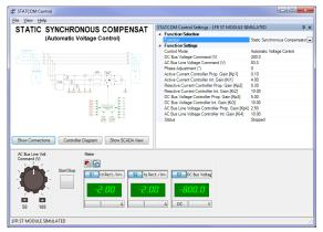
The Static Synchronous Compensator (STATCOM) Control Function Set enables the following devices required for the study of STATCOMs to be implemented using the Data Acquisition and Control Interface, and the IGBT Chopper/ Inverter:
