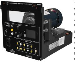
The Four-Quadrant Dynamometer/Power Supply is a highly versatile USB peripheral designed to be used in the Electric Power Technology Training Systems. Two operating modes are available: Dynamometer and Power Supply. A wide variety of user-selectable functions is available in each operating mode.
