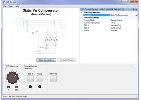
The Static Var Compensator (SVC) Control Function Set enables the following devices required for the study of SVCs to be implemented using the Data Acquisition and Control Interface, and the Power Thyristors:
