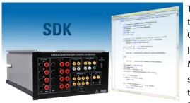
The DACI SDK (Software Development Kit) offers the possibility to control various inputs and outputs of the Data Acquisition and Control Interface using third-party rapid prototyping software like Mathworks<sup>®</sup> MATLAB, National Instruments<sup>®</sup> LabVIEW, Microsoft Visual Studio and other programming tools that support Microsoft<sup>®</sup> .NET Framework 4.0. The SDK gives users the possibility to build their own advanced functions using the Data Acquisition and Control Interface.
