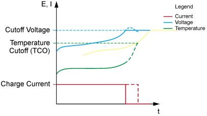
Ni-MH Battery Charger (Constant-Current Charge with Voltage Cutoff and TCO), Model 8968-5
