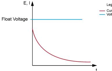
Legend This function uses the four-quadrant Current power supply to implement a lead-acid battery float charger. This charger applies a constant voltage to the battery. The user only has to specify the battery float charging voltage. The function indicates the voltage, current, and electrical power at the charger output. The Lead-Acid Battery Float Charger function is well suited to charge several lead-acid batteries connected in parallel overnight so they are ready for next-day lab sessions.
