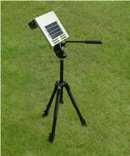
Monocrystalline Silicon Solar Panel installed on a tripod (setup for outdoor exercises).
