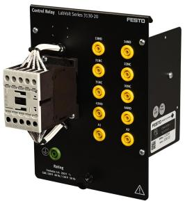
The Control Relay is a general purpose, industrial-type relay with two sets of normally open (NO) contacts and two sets of normally closed (NC) contacts.
