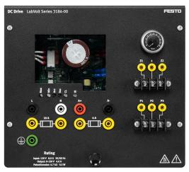
The DC Drive consists of a pulse-width modulated (PWM) dc motor speed control with maximum and minimum speed, current limitation, and IR compensation adjustments. Some electrical connections can be made using either the banana jacks or the terminal blocks.
