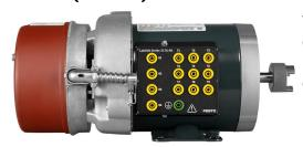
The Brake Motor consists of a three-phase, four-pole, squirrelcage induction motor equipped with a spring set brake for holding and stopping (fail-safe). The motor is dual voltage and can operate at either a low-voltage or a high-voltage setting.
