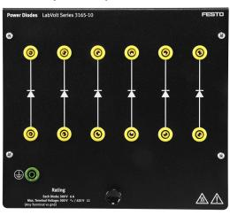
The Power Diodes module consists of six silicon rectifier diodes. The anode and cathode of all diodes are wired to independent front panel terminals, thereby allowing the diodes to be connected in any single-phase and three-phase rectifier configuration.
