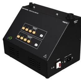
The Servo Controller incorporates a state-of-the-art 32-bit microcontroller coupled to a power amplifier specially designed for brushed and brushless dc motor control. The Servo Controller connects to a host computer via a USB connection and is fully configurable for various types of open- and closed-loop control applications. The controller allows three methods of control:
