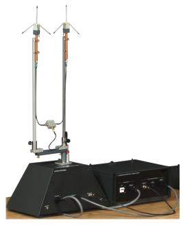
The Two Element Phasing Kit consists of an additional drooping monopole antenna (one is already included in the ATMS), an additional antenna mast with vertical mounting clips (one is already included in the ATMS), a power splitter/combiner, and a set of RF cables of different lengths. Phase shifts of 0, 90, and 180 degrees can be produced with the supplied RF cables. Other phase shifts can be produced by using RF cables having lengths that differ from those of the supplied RF cables.
