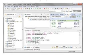
Through a USB port with a computer, a Windows-based software (debugger) allows for a direct interraction with the program DSP registers, memory, and peripherals.
