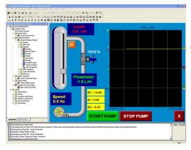
FactoryTalk View ME Station (Commercial) is a Windows-based application, produced by Rockwell Software, allowing the creation of graphic interfaces for the Touch Screen Graphic Terminal, Model 5922. Using programs developed with FactoryTalk View ME Station (Commercial), data available over the network can be displayed on the screen and commands can be sent over the Ethernet network.
