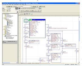
Studio 5000 Logix Designer is a Windows-based application, produced by Rockwell Software™, used to build programs for CompactLogix PLCs.
