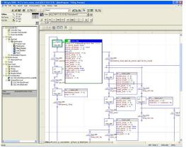
Studio 5000 Logix Designer is a Windows-based application, produced by Rockwell Software™, used to build programs for PLCs.
