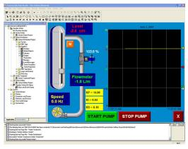
FactoryTalk View ME Station is a Windows-based application, produced by Rockwell Software, allowing the creation of graphic interfaces for the Touch Screen Graphic Terminal, Model 5922. Using programs developed with FactoryTalk View ME Station, data available over the network can be displayed on the screen and commands can be sent over the Ethernet network.
