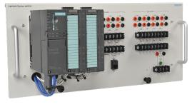
The Programmable Logic Controller (S7-1516) consists of a controller from the Siemens family. This powerful PLC comes with sixteen 24 V dc inputs, eight 4-20 mA inputs, eight 24 V dc output relays and eight 4-20 mA outputs hardwired to both banana jacks and terminal blocks on the module front panel. Banana jacks provide an easy and fast way to wire a setup, while terminal blocks allow students to wire their setup in a way much closer to what is commonly found in the industry.
