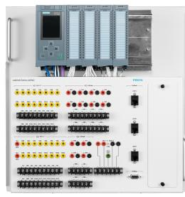
The Programmable Logic Controller (S7-1516) consists of a controller from the Siemens family. This powerful PLC comes with sixteen 24 V dc inputs, eight 4-20 mA inputs, eight 24 V dc output relays and eight 4-20 mA outputs hardwired to both banana jacks and terminal blocks on the module front panel. Banana jacks provide an easy and fast way to wire a setup, while terminal blocks allow students to wire their setup in a way much closer to what is commonly found in the industry.
