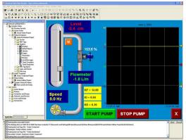
FactoryTalk View Studio ME (Commercial) is a Windows-based application, produced by Rockwell Software, allowing the creation of graphic interfaces for the Touch Screen Graphic Terminal, Model 5922. Using programs developed with FactoryTalk View Studio ME (Commercial), data available over the network can be displayed on the screen and commands can be sent over the Ethernet network.
