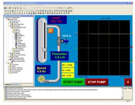
FactoryTalk View Studio ME is a Windows-based application, produced by Rockwell Software, allowing the creation of graphic interfaces for the Touch Screen Graphic Terminal, Model 5922. Using programs developed with FactoryTalk View Studio ME, data available over the network can be displayed on the screen and commands can be sent over the Ethernet network.
