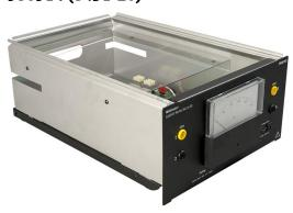
The Single-Phase Wattmeter is used to indicate active power in single-phase circuits. Its electronic design uses voltage and current sensors to sample line voltage and current. Voltage and current circuits are internally connected so that students only have to connect the "line" and "load" terminals of the module.
