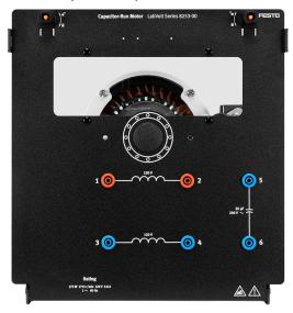
The Capacitor-Run Motor is fitted with a running capacitor and running windings that are independently terminated and identified on the faceplate to facilitate experimentation of various machine connections, including operation from a two-phase source of power. The design of the machine has been optimized so that it operates like a two-phase motor at full load when connected to a single-phase source.
