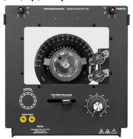
The Electrodynamometer is made of a squirrel-cage rotor fitted in a dc-excited stator. Mechanical loading is achieved by increasing the stator field current, which generates eddy currents in the driven rotor. The stator is trunnion-mounted on ball bearings and rotates against a helicoidal spring to oppose braking torque.
