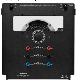
The Four-Pole Squirrel-Cage Induction Motor is a 0.2 kW squirrel-cage induction machine mounted in a full-size EMS module. The machine stator windings are independently connected (six jacks), allowing connection in either wye or delta configuration. Connections to the machine are made through color-coded safety banana jacks located on the front panel on the module.
