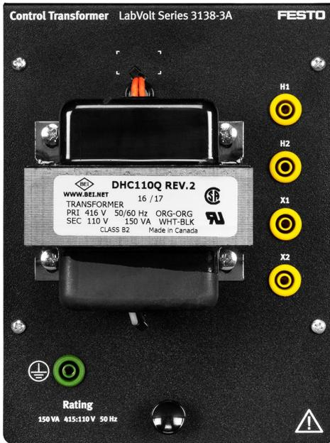
The Control Transformer converts the ac power network voltage (e.g., 208 V, 380 V, 415 V) to 110/120 V. The primary windings of the transformer are fuse-protected to prevent damage to the equipment.
