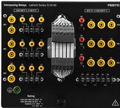
The Interposing Relays module consists of a bidirectional voltage converter for high and low control voltages. This model is equipped with three relays with 24 V dc coils and three relays with 110/120 V ac coils. Electrical connections for the low-voltage coils and contacts can be made using either the banana jacks or the terminal blocks.
