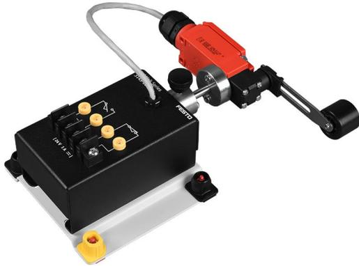
The Limit Switch consists of a limit switch with two contacts, one normally open and one normally closed. The model can be used directly with the Reversible AC Motor, Model 3174-3, and become part of its mechanism.
