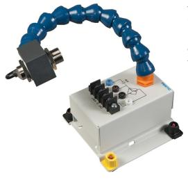
The Inductive Proximity Switch is sensitive to metals. The sensor is mounted on a flexible support for easy positioning. The model has one normally open and one normally closed contact, and the electrical connections are made using either the banana jacks or the terminal block.
