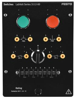
The Switches module consists of two general-purpose push buttons, one green with a normally open contact and one red with a normally closed contact, and a three-position, single-pole selector switch. Electrical connections can be made using either the banana jacks or the terminal block.
