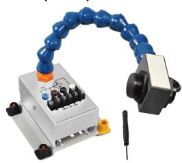
The Capacitive Proximity Switch is sensitive to every material. The sensor is mounted on a flexible support for easy positioning. The model has one normally-open and one normally-closed contact, and the electrical connections are made using either the banana jacks or the terminal block.
