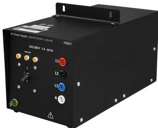
The AC Power Supply provides ac power for the Industrial Controls Training System. The outlet is fed from a three-phase, four-wire breaker panel supplied elsewhere. The power supply contains input and output pilot lamps, two "on-off" switches and dual sets of four color-coded banana jacks for three-phase voltage. All outputs are circuit-breaker protected. The AC Power Supply mounts on the upper shelf of the Mobile Workstation, Model 3103-4, and can provide power to both sides of the workstation.
