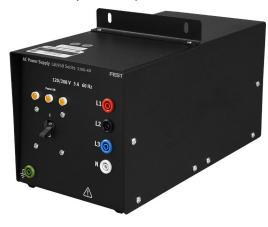
The AC Power Supply provides ac power for the Industrial Controls Training System. The outlet is fed from a three-phase, four-wire breaker panel supplied elsewhere. The power supply contains input and output pilot lamps, two "on-off" switches and dual sets of four color-coded banana jacks for three-phase voltage. All outputs are circuit-breaker protected. The AC Power Supply mounts on the upper shelf of the Mobile Workstation, Model 3103-4, and can provide power to both sides of the workstation.
