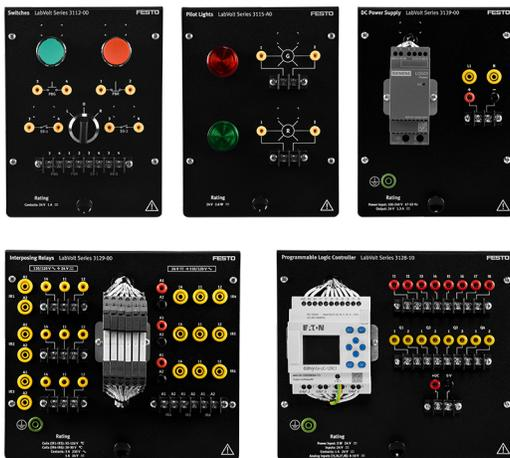
The Programmable Logic Controller Training System introduces students to the use of PLCs for motor control.
