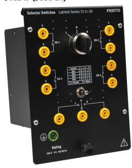
The Selector Switches module consists of a three-position, two-pole selector switch and a single-pole double-throw toggle switch. It allows the user to alternate between two control circuit branches through the selector (at the top) or the toggle (at the bottom) switches. The two switches work independently. Selecting a position activates or deactivates the maintained contacts.
