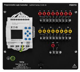
The Programmable Logic Controller consists of a small controller programmed in four different languages (ST, FBD, LD, EDP) with eight inputs (24 V dc), four of them can be turned into analog inputs (0-10 V dc), and four relay outputs. The programming is done using the LCD screen and the keypad on the controller or using the programming software (easySoft) and cable included in this model. Electrical connections can be made using either the banana jacks or the terminal blocks.
