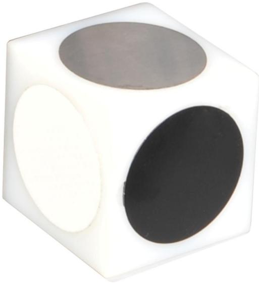
The Reflective Block consists of a block with various types of reflection surfaces: white, black, shiny metallic, matte black metallic, and retroreflective. The dimensions of the block are: 75 x 75 x 75 mm (3 x 3 x 3 in).
