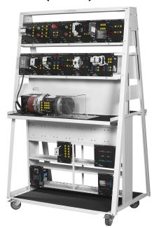
The Industrial Controls Training Systems are designed to teach the theory and techniques of electric motor controllers. They allow students to select and mount control devices to form typical control circuits, and to troubleshoot them once a fault is inserted. The systems offer unique controls training possibilities, are modular, and include insertable faults.
