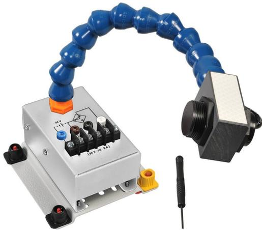
The Capacitive Proximity Switch is sensitive to every material. The sensor is mounted on a flexible support for easy positioning. The model has one normally-open and one normally-closed contact, and the electrical connections are made using either the banana jacks or the terminal block.
