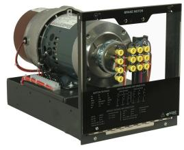
The Brake Motor (EMS Version) consists of a three-phase, four-pole, squirrel-cage induction motor equipped with a spring-set brake for holding and stopping (fail-safe). The motor is dual voltage and can operate at either a low-voltage or a high-voltage setting.
