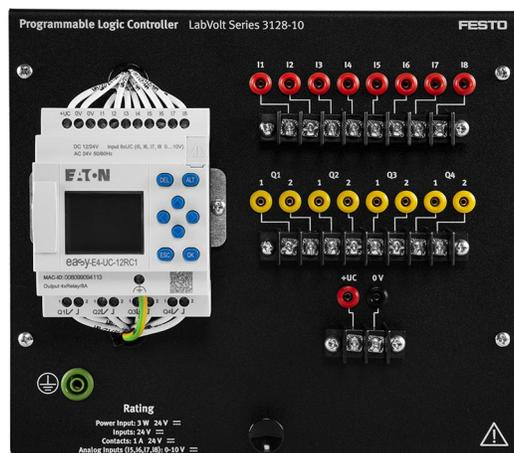
The Programmable Logic Controller consists of a small controller programmed in four different languages (ST, FBD, LD, EDP) with eight inputs (24 V dc), four of them can be turned into analog inputs (0-10 V dc), and four relay outputs. The programming is done using the LCD screen and the keypad on the controller or using the programming software (easySoft) and cable included in this model. Electrical connections can be made using either the banana jacks or the terminal blocks.
