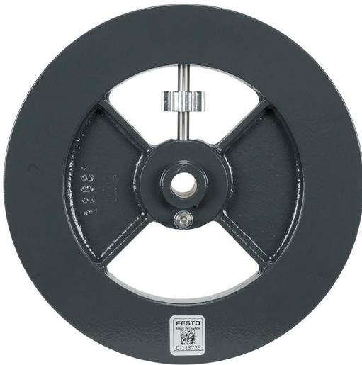
The balanced Inertia Wheel securely attaches to any 0.2 kW machine. When the inertia wheel is rotated at 1800 r/min, it stores 790 joules of energy (550 joules at 1500 r/min).
