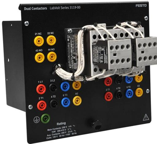
The Dual Contactors module consists of two mechanically interlocked, three-pole contactors with two auxiliary contacts. Each contactor also comes with three additional auxiliary contacts, not wired to the front panel, for direct connection with other devices.
