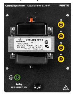
The Control Transformer converts the ac power network voltage (e.g.,  $208\,V$ ,  $380\,V$ ,  $415\,V$ ) to  $110/120\,V$ . The primary windings of the transformer are fuse-protected to prevent damage to the equipment.
