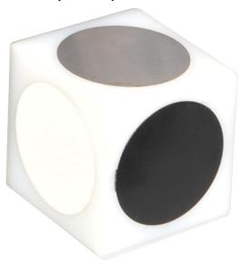
The Reflective Block consists of a block with various types of reflection surfaces: white, black, shiny metallic, matte black metallic, and retroreflective. The dimensions of the block are: 75  $\times$  75  $\times$  75 mm (3  $\times$  3  $\times$  3 in).
