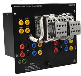
The Dual Contactors module consists of two mechanically interlocked, three-pole contactors with two auxiliary contacts. Each contactor also comes with three additional auxiliary contacts, not wired to the front panel, for direct connection with other devices.
