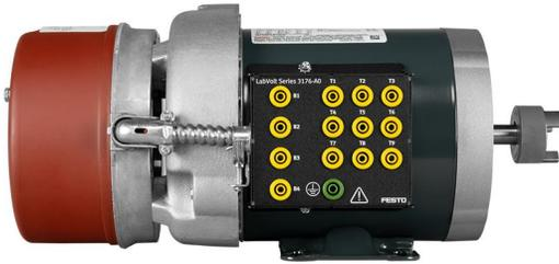
The Brake Motor consists of a three-phase, four-pole, squirrel-cage induction motor equipped with a spring set brake for holding and stopping (fail-safe). The motor is dual voltage and can operate at either a low-voltage or a high-voltage setting.
