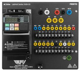
The AC Drive consists of a variable frequency speed drive with V/Hz control. The AC Drive has programmable
