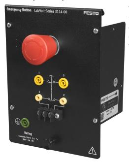
The Emergency Button consists of an emergency push button with two sets of contacts, both normally closed, that can be used to control devices operating at low and high voltages. Electrical connections for the low-voltage contact can be made using either the banana jacks or the terminal block.
