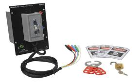
The Lockout Module consists of a lockable three-phase disconnect switch. The lockout device is a six-lock scissor type and the disconnect switch is a three-pole unit. Three padlocks and three identification tags are also included. One module is required for single-sided stations, while two are required for double-sided stations.
