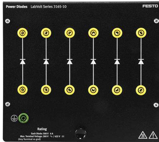
The Power Diodes module consists of six silicon rectifier diodes. The anode and cathode of all diodes are wired to independent front panel terminals, thereby allowing the diodes to be connected in any single-phase and three-phase rectifier configuration.
