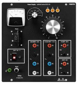
The Power Supply module is the primary component of the system. All associated equipment is powered by this power supply. A flexible, 5-wire power cord, terminated with a 5-prong, twist-lock plug and line cap, feeds the module. A mechanical interlock on the line cap prevents the removal of an energized Power Supply from its locked position in the workstation. The Power Supply requires a 3-phase, wye-connected, 5-wire service installation including ground and neutral.
