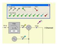
Probes can be dragged from the Probes bar and connected to circuit Test Points (TPs) in order to observe signals using the virtual instruments.
