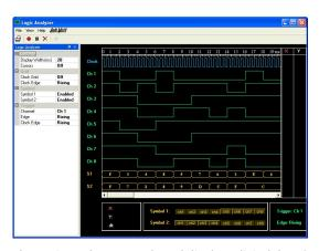
The Logic Analyzer records and displays digital data from multiple test points.
