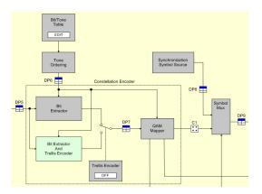
The ADSL application performs constellation encoding with or without Trellis Coding and allows modifying the number of bits allocated to each tone (subcarrier).
