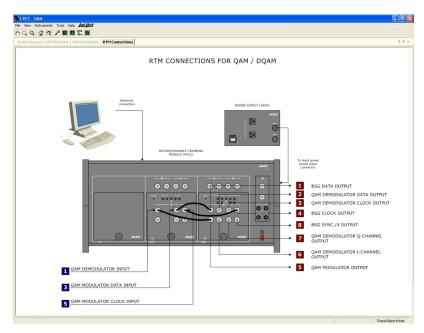
The RTM Connections diagram identifies the RTM inputs and outputs and shows the external connections.
