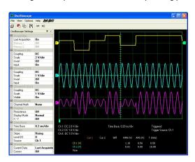
The virtual Oscilloscope allows observation and measurement of analog and digital signals.
