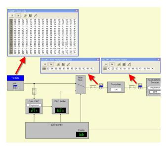
Data Points are provided where digital data is present in a circuit. Doubleclicking a Data Point opens a table displaying the data as decimal or hexadecimal values.
