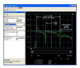
The Spectrum Analyzer displays frequency spectra, such as this spectrum of an ADSL signal.
