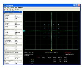
In the X-Y mode, the Oscilloscope can display the signal constellation, such as this 16-QAM constellation.
