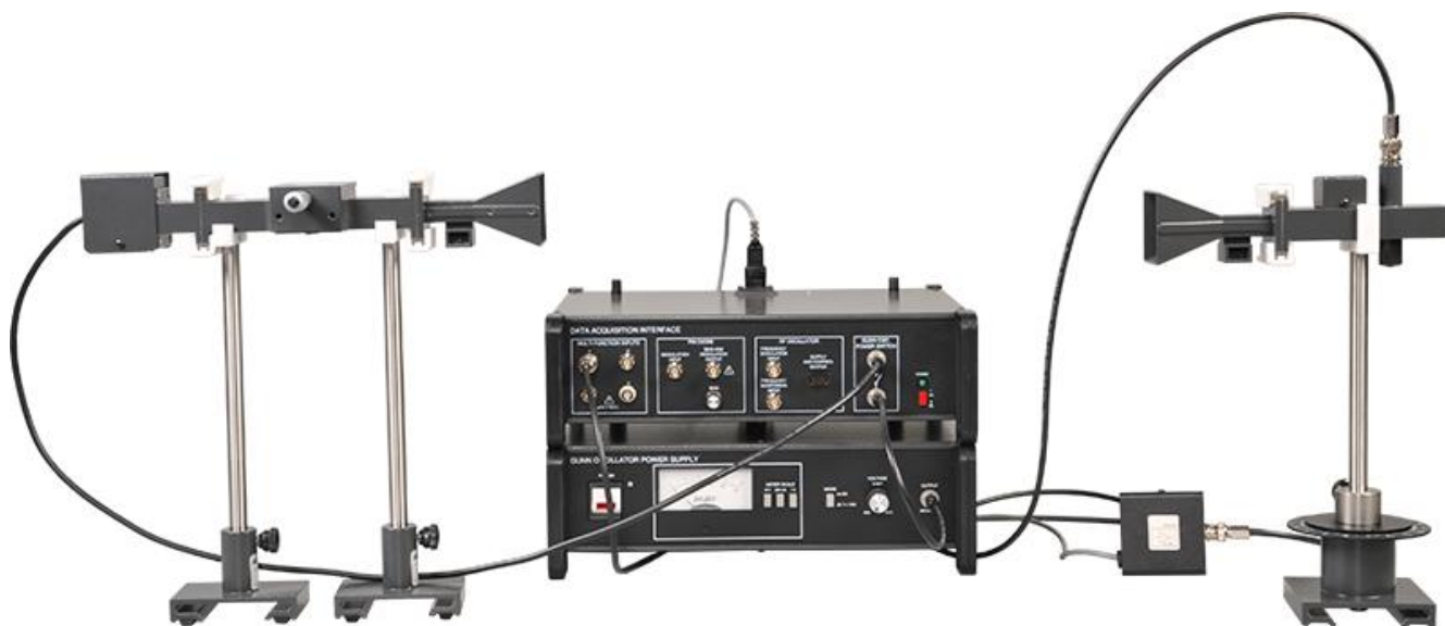
Wireless transmission of a microwave signal [typical distance between the antennas: 40 cm (16 in)].
