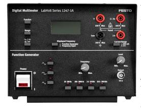
The Digital Multimeter / Function Generator is a compact, general-purpose instrumentation module that provides the necessary test equipment (except the oscilloscope) to perform the courses in the FACET program. The module consists of a sine/square/triangle waveshape function generator and an auto-ranging digital multimeter. All instruments share a common power input and are housed in a portable enclosure.
