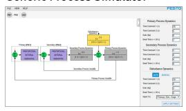
The generic process simulator provides simplified simulation to introduce basic concepts of process control. The simulator can be configured as first or second order process, with or without dead time. The disturbance can be configured as first order. The process and disturbance have variable gains.
