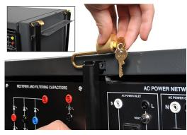
The EMS modules are guided into position along stainless steel guide rails. Separators between each bay of the workstation ensure perfect alignment of the EMS modules and allow their easy insertion in the workstation. A holding mechanism ensures that each EMS module stays in place once it is installed in a compartment of the workstation. A front-mounted push lever allows all EMS modules on the workstation to be
