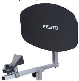
The Radar Antenna mounts on the rotating-antenna pedestal and has a miniature plug-in connector for quick RF coupling. It uses an offset-feed design to reduce masking effects. A screen of microwave-radiation-absorbing material is also supplied, which, although not required due to the low level of RF power radiated by the system, provides training in microwave safety techniques.
