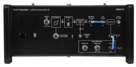
The Radar Transmitter is an instructional module designed to provide training in system- and module-level troubleshooting. It has switches that the instructor can use to insert faults. These switches, as well as the circuit boards and test points, are accessed through the hinged door on top of the module.
