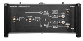
The Radar Receiver is an instructional module designed to provide training in system- and module-level troubleshooting. It has switches that the instructor can use to insert faults. These switches, as well as the circuit boards and test points, are accessed through the hinged door on top of the module.
