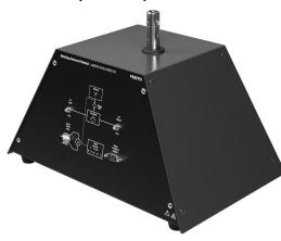
The Rotating-Antenna Pedestal is the mount and drive motor for the radar antenna. It provides the RF connection between the antenna and the radar transmitter and receiver. Antenna position feedback is obtained from an incremental optical shaft encoder, the output of which may be monitored through front-panel test points. The RF section includes a circulator for simultaneous transmission and reception. A rotary joint provides RF coupling to the rotating antenna mount.
