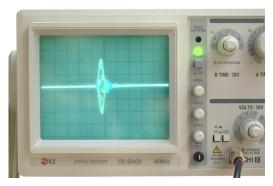
An oscilloscope is required for target echo visualization on an A-scope display as well as time-domain observation of signals at outputs and test points (the Model 797 Dual Trace Oscilloscope is recommended).
