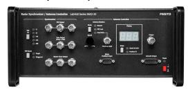
The Radar Synchronizer / Antenna Controller is used for Pulse Repetition Frequency (PRF) generation and synchronization of the radar system. It also controls the operating parameters of the radar antenna.
