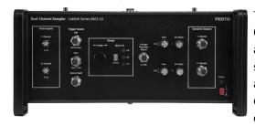
The Dual-Channel Sampler performs time expansion of the I- and Q-channel baseband signals from the radar receiver in order to allow further processing and display. It has three switches to select the system observation range, as well as control knobs for adjusting the system range origin, the balance of the I- and Q-channel output signals, and the DC offsets at the I- and Q-channel outputs. A time base output is provided to obtain an A-scope display on a conventional oscilloscope.
