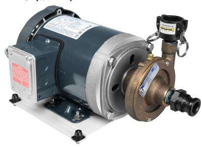
The Motor and Pump Assembly (Multiple-Pump) consists of a mounting base, a motor, and a centrifugal pump directly mounted to the motor frame. The assembly is designed to be secured to the perforated worksurface.
