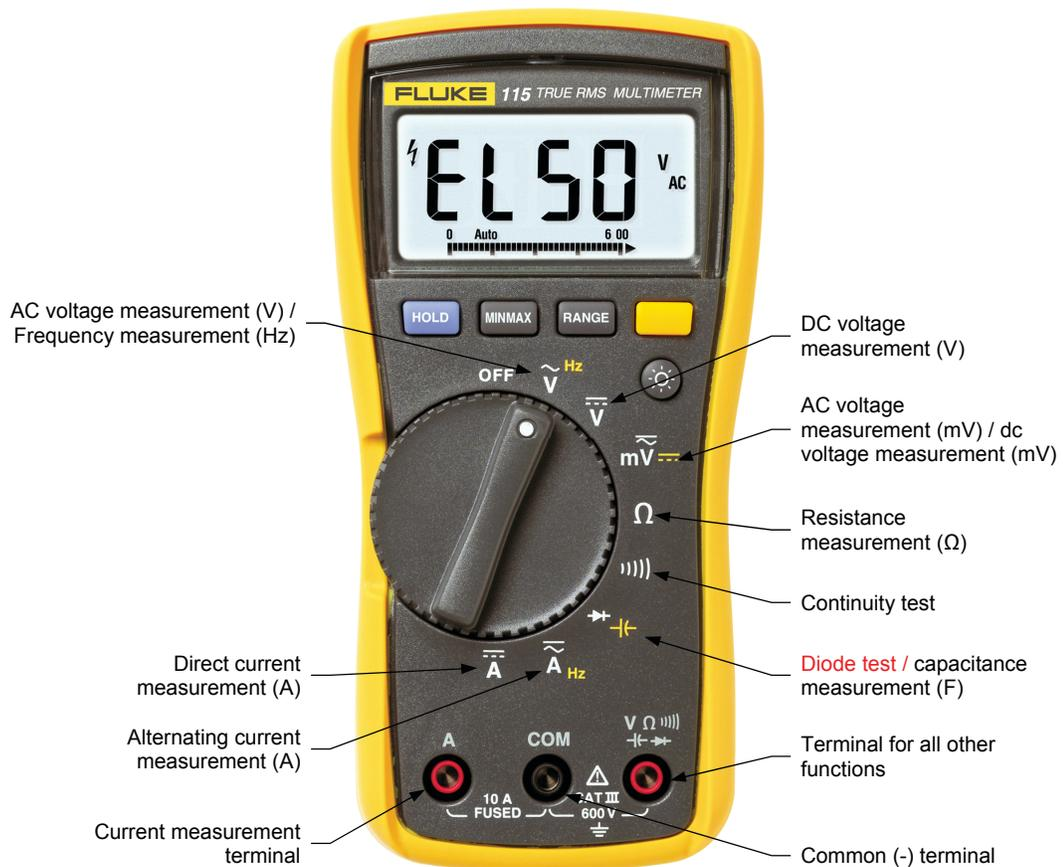
Figure 10. Typical multimeter.
