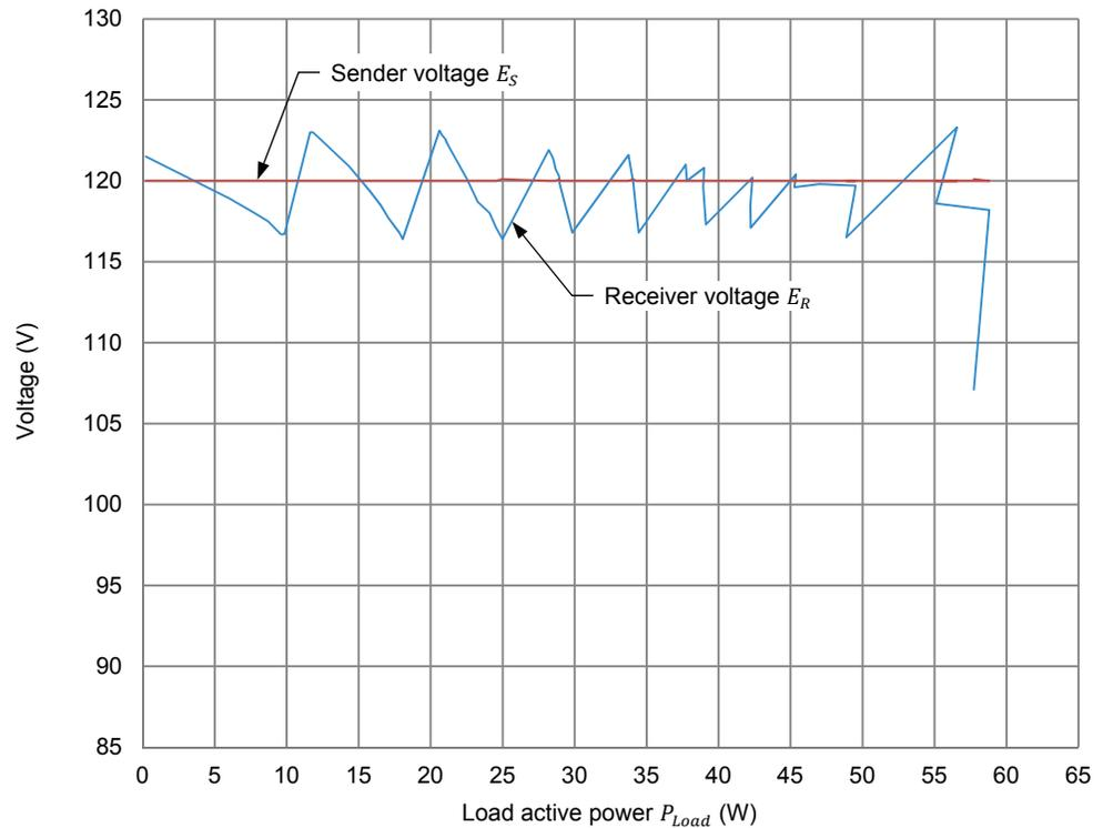
Power-voltage curve of the 700 km (about 435 miles) ac transmission line (for one phase) when distributed SSC (inductive and capacitive) is used for voltage compensation.
