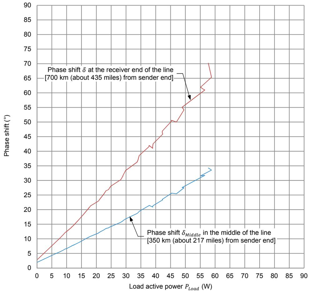
Phase shift  $\delta$  between voltages  $E_R$  and  $E_S$  and phase shift  $\delta_{Middle}$  between voltages  $E_{Middle}$  and  $E_S$  as a function of the active power  $P_{Load}$  when the 700 km (about 435 miles) ac transmission line is voltage compensated using distributed SSC (inductive and capacitive).
