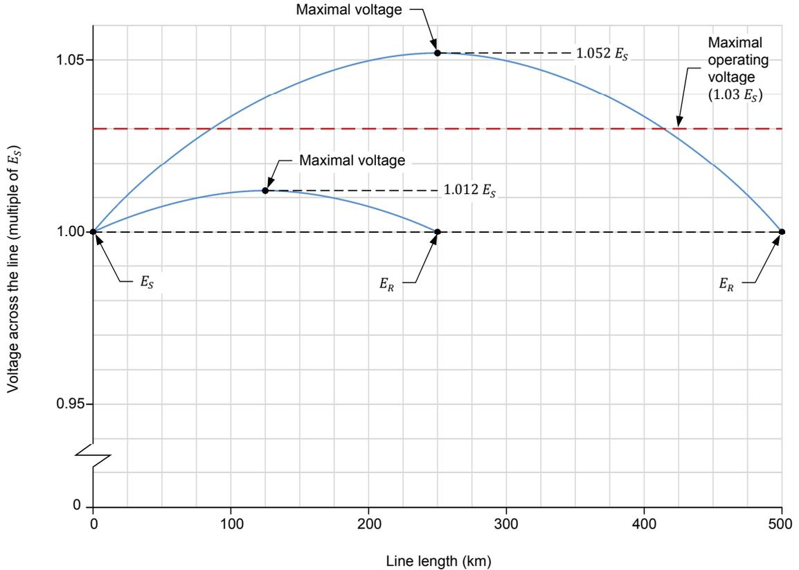
**Figure 45.** Voltage profiles along the 250 km (155 miles) and 500 km (310 miles) ac transmission lines shown in the discussion of Exercise 4 when they are voltage compensated using switched shunt compensation at both ends and operate without load.
