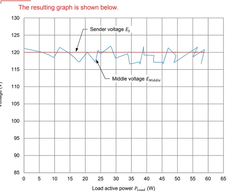
Power-voltage curve in the middle of the 700 km (about 435 miles) ac transmission line (for one phase only) when distributed SSC (inductive and capacitive) is used for voltage compensation.
