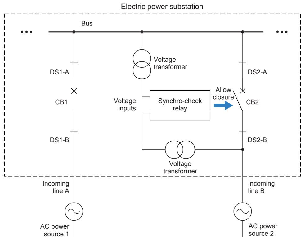
Figure 33. A synchro-check relay is used to check the synchronism of ac power sources before allowing closure of an incoming line circuit breaker.
