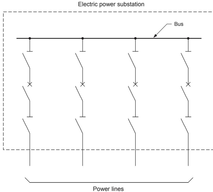
Figure 25. Single-line diagram of an electric power substation implemented using the single bus scheme.
