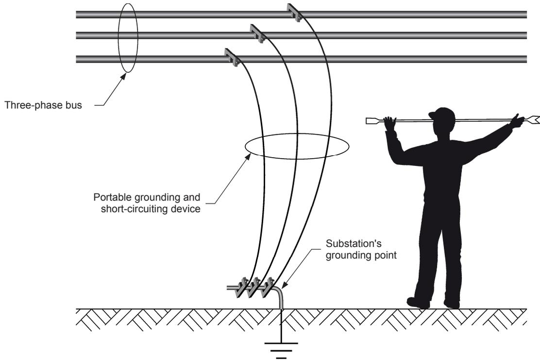
Figure 30. A portable grounding and short-circuiting device installed on a bus in an electric power substation.
