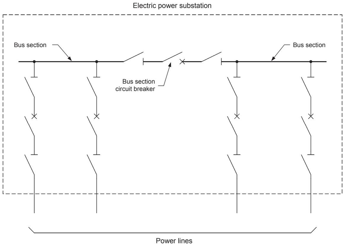
Figure 26. Single-line diagram of an electric power substation implemented using the single bus scheme with bus section circuit breakers.
