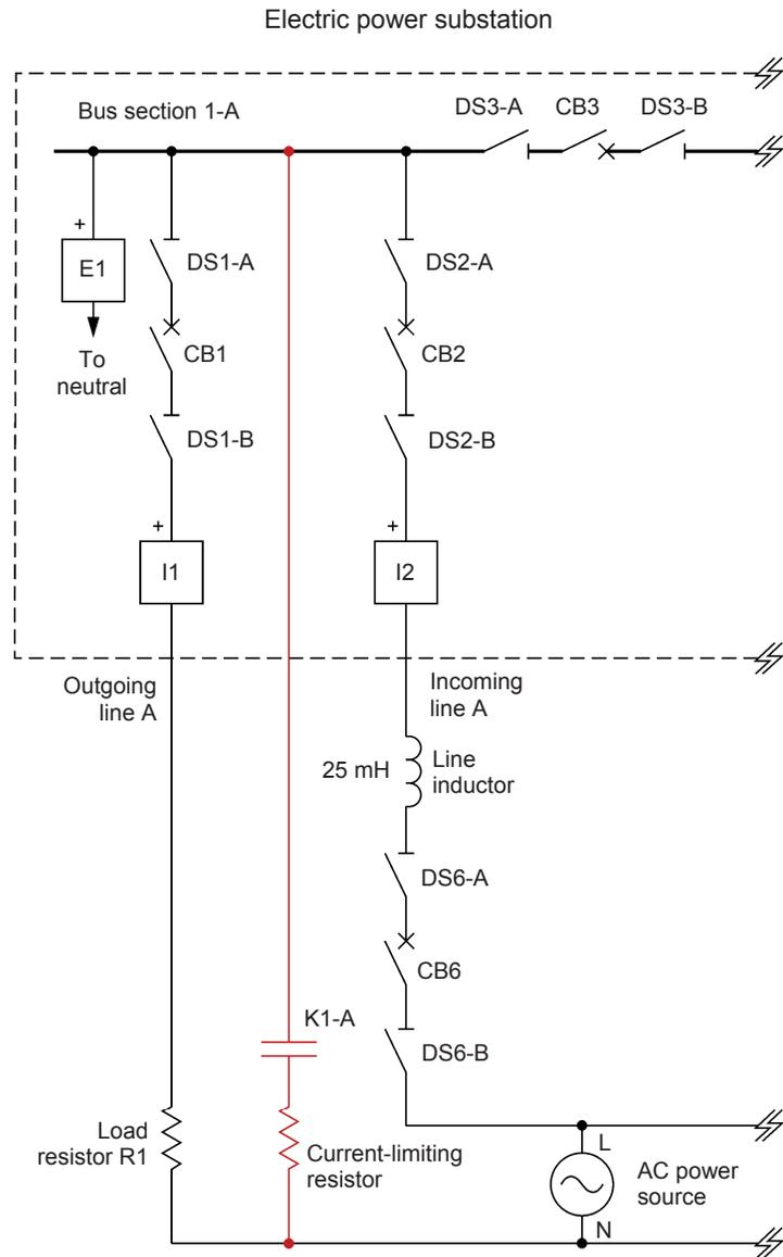
Figure 38. Connection of the Fault Module required to insert a fault at bus section 1-A of the electric power substation.
