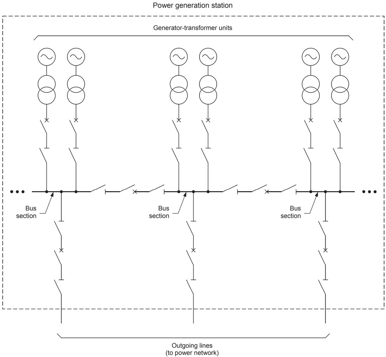
Figure 28. Single-line diagram of a large power generation station using the single bus scheme with bus section circuit breakers to interconnect generator-transformer units to the outgoing lines.
