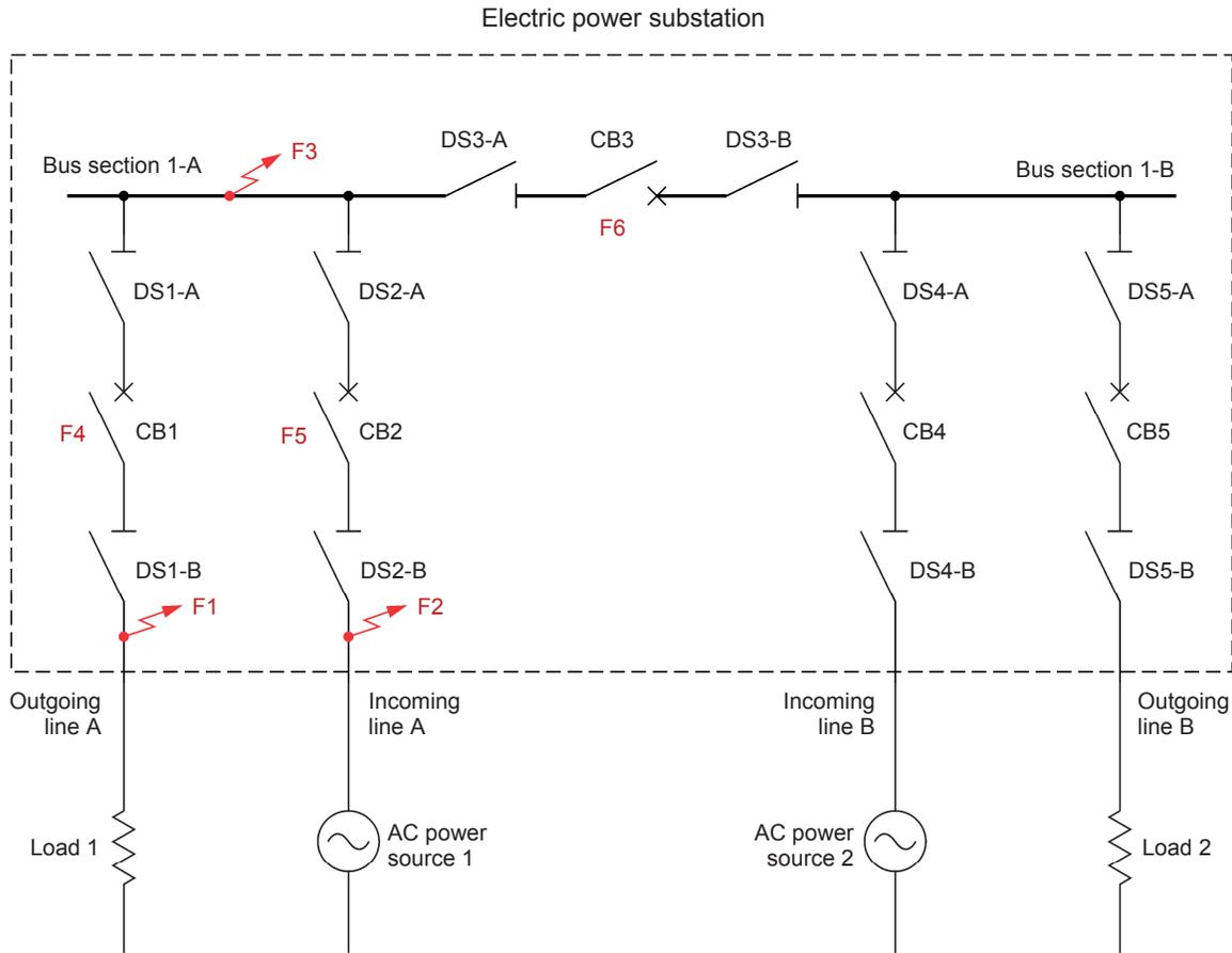
Figure 27. Faults at various locations in a substation implemented using the single bus scheme with bus section circuit breakers.
