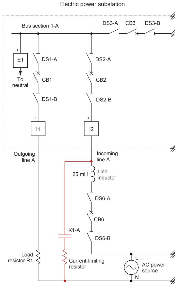
Figure 37. Connection of the Fault Module required to insert a fault at incoming line A of the electric power substation.
