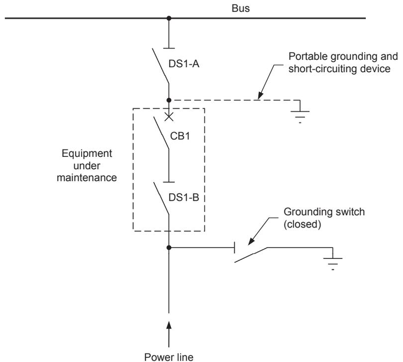
Figure 29. Grounding switch and portable grounding and short-circuiting device used to achieve protective grounding in an electric power substation.
