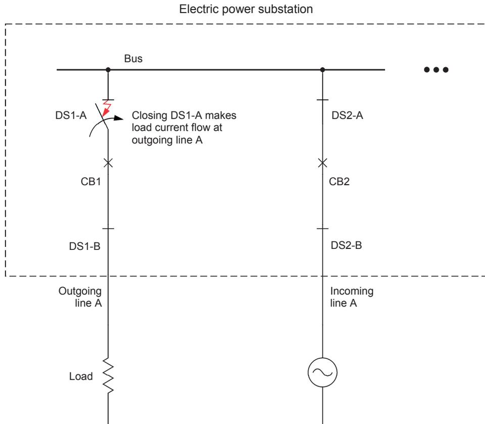
**Figure 32. Closing a disconnecting switch while the corresponding circuit breaker is closed should be avoided.**
