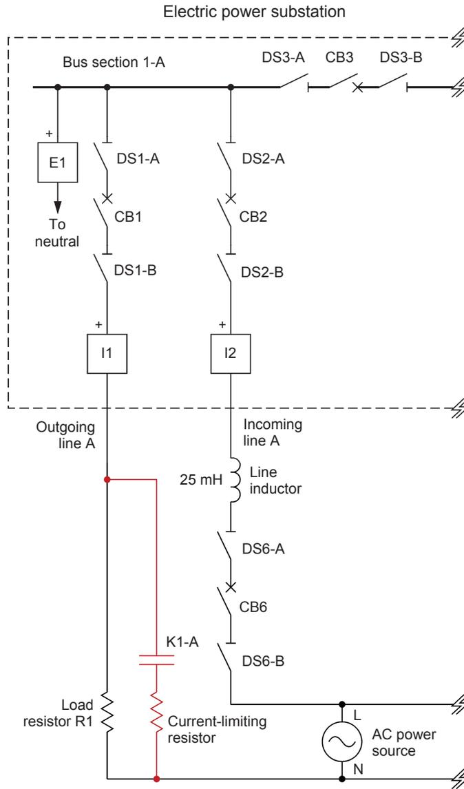
Figure 36. Connection of the Fault Module required to insert a fault at outgoing line A of the electric power substation.
