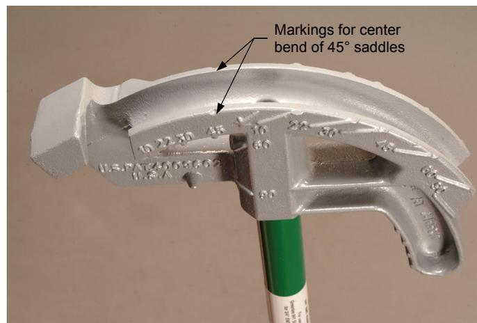
**Figure 30.** Markings on the bending shoe of a typical hand bender (GreenLee® Site-Rite II® 841) that are used when performing the center bend of a saddle.
