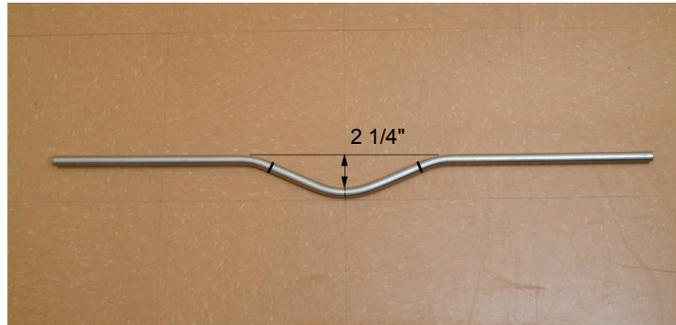
**Figure 31.** A three-bend saddle deep enough to clear a 2 1/4" obstruction (performed on a piece of 1/2" EMT).
