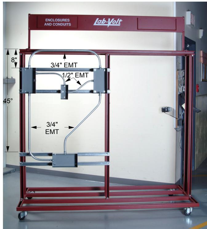
Figure 36. Dummy enclosures and box interconnected with 1/2" and 3/4" EMT.
