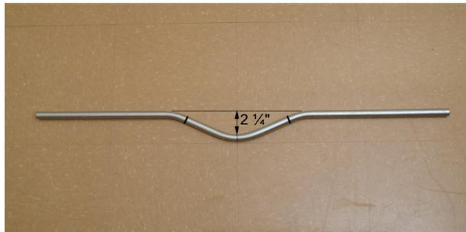
**Figure 40.** A three-bend saddle deep enough to clear a 2 1/4" obstruction (performed on a piece of 1/2" EMT).
