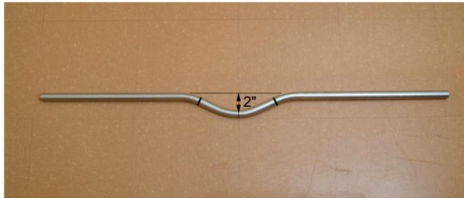
Figure 47. A three-bend saddle deep enough to clear a 2" obstruction (performed on a piece of 3/4" EMT).
