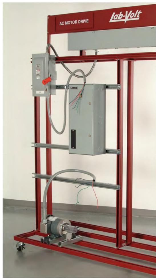
**Figure 2-1.** New MCE installed on the Mobile Workstation.
