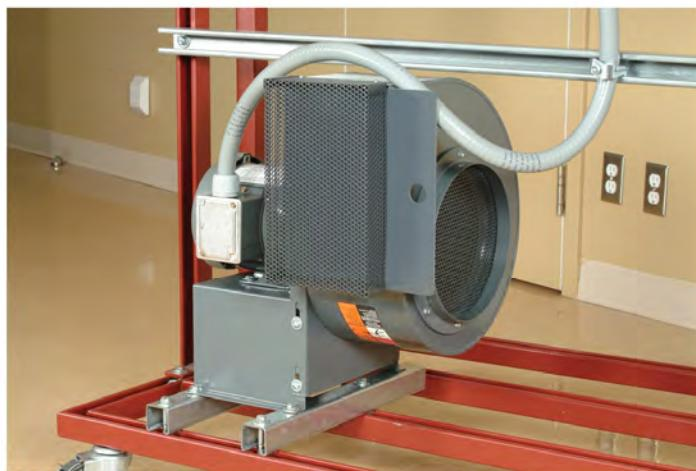
**Figure 2-7. Blower installed on the lower horizontal rails of the Mobile Workstation.**
