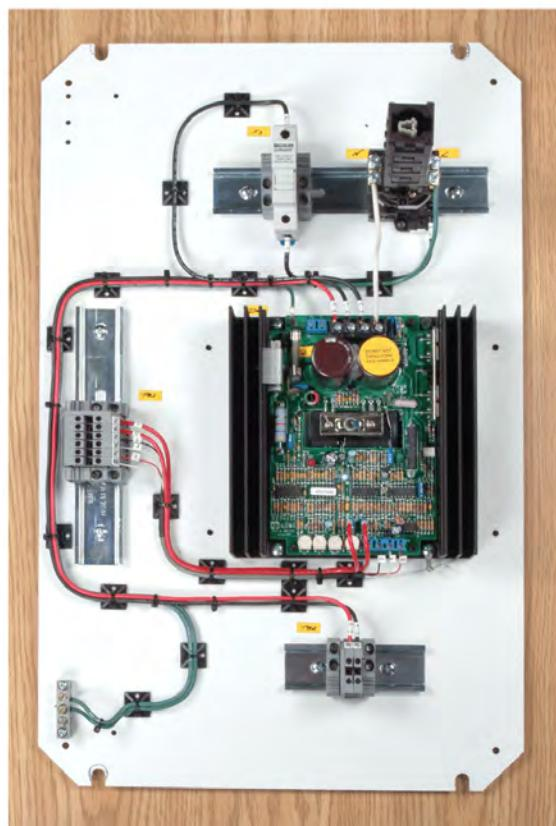
Figure 1-2. Assembled DC motor drive (MCE mounting plate).
