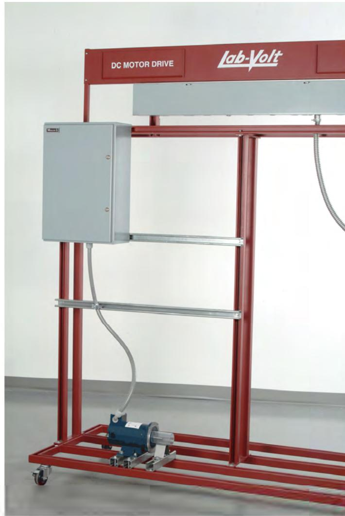
Figure 1-4. The DC motor drive with all conduits installed except the one that goes to the wiring trough of the system's three-phase power bus.
