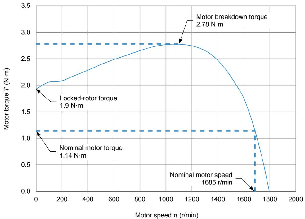
Three-phase induction motor torque  $T$  (expressed in N·m) as a function of the motor speed  $n$ .
