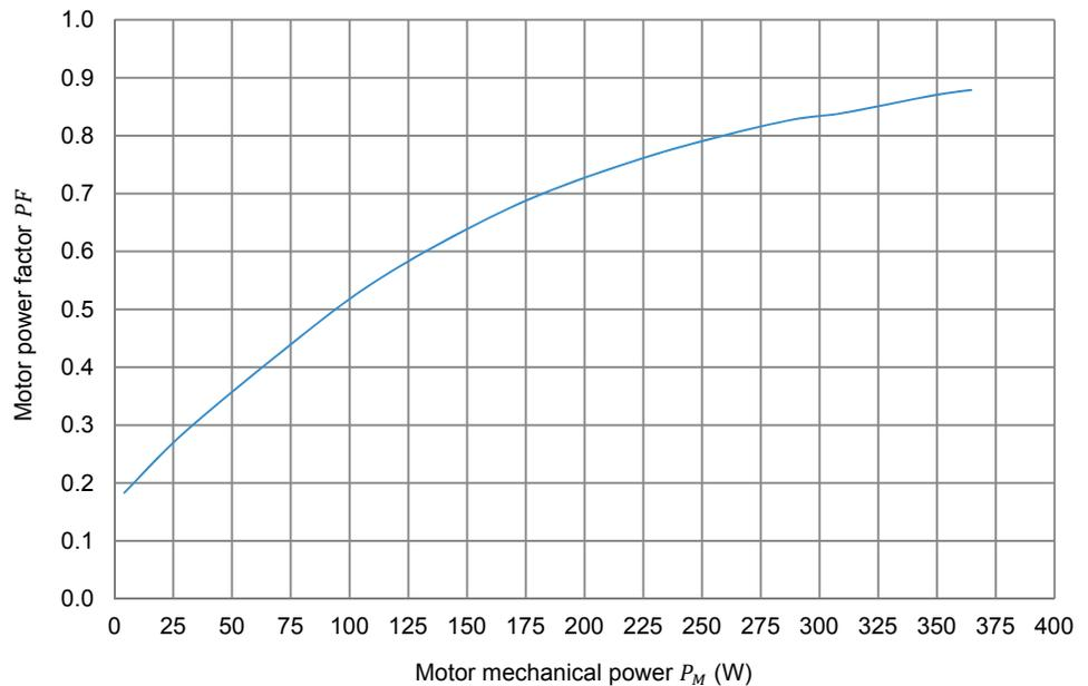
Three-phase induction motor power factor  $PF$  as a function of the motor mechanical power  $P_M$ .
