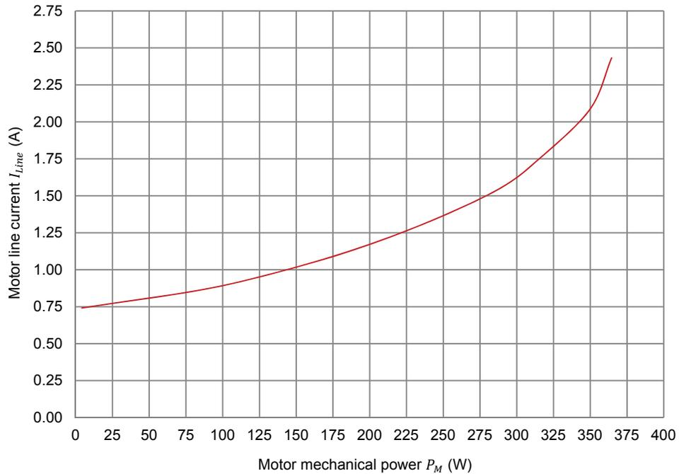
Three-phase induction motor line current  $I_{Line}$  as a function of the motor mechanical power  $P_M$ .
