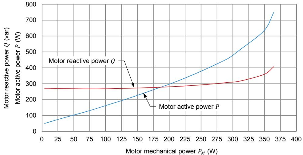
Three-phase induction motor active power  $P$  and reactive power  $Q$  as a function of the motor mechanical power  $P_M$ .
