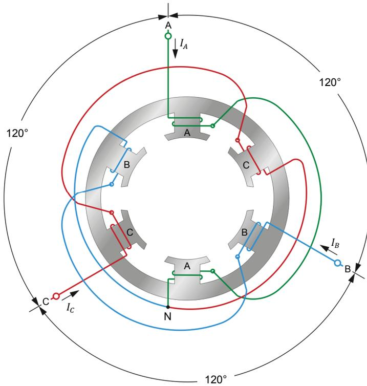
Figure 2-5. Three-phase stator windings (two poles per phase).
