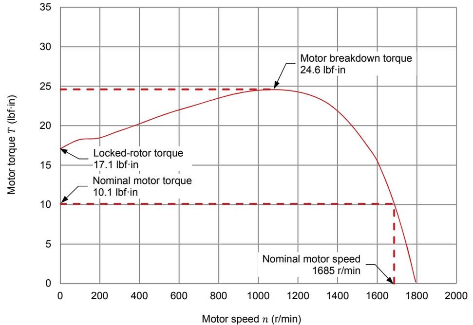
Three-phase induction motor torque  $T$  (expressed in lbf·in) as a function of the motor speed  $n$ .
