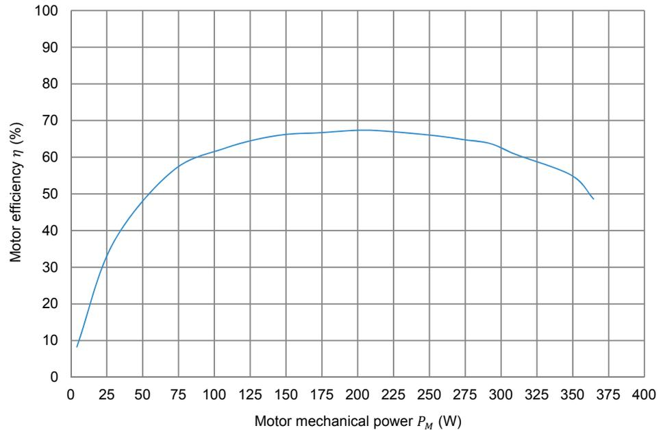
Three-phase induction motor efficiency  $\eta$  as a function of the motor mechanical power  $P_M$ .
