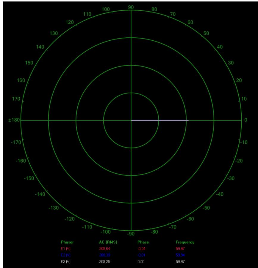
Phasors of the voltage  $E_{Reg,A}$  at region A, the modified voltage  $E'_{Reg,A}$  at region A, and the voltage  $E_{Reg,B}$  at region B when the Regulating Autotransformer is set to a 0° phase shift.
