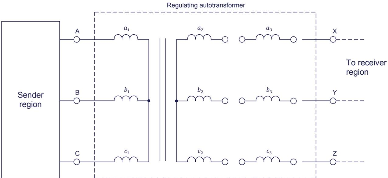
Figure 38. Equivalent circuit of a regulating autotransformer.
