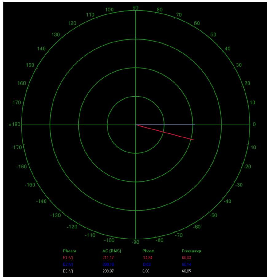
Phasors of the voltage  $E_{Reg,A}$  at region A, the modified voltage  $E'_{Reg,A}$  at region A, and the voltage  $E_{Reg,B}$  at region B when the Regulating Autotransformer is set to a  $-15^\circ$  phase shift.
