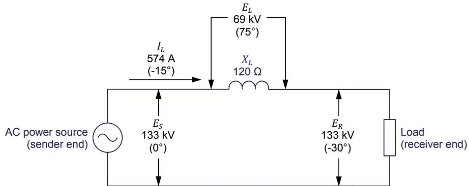
Figure 32. Voltage-compensated 230 kV ac transmission line.
