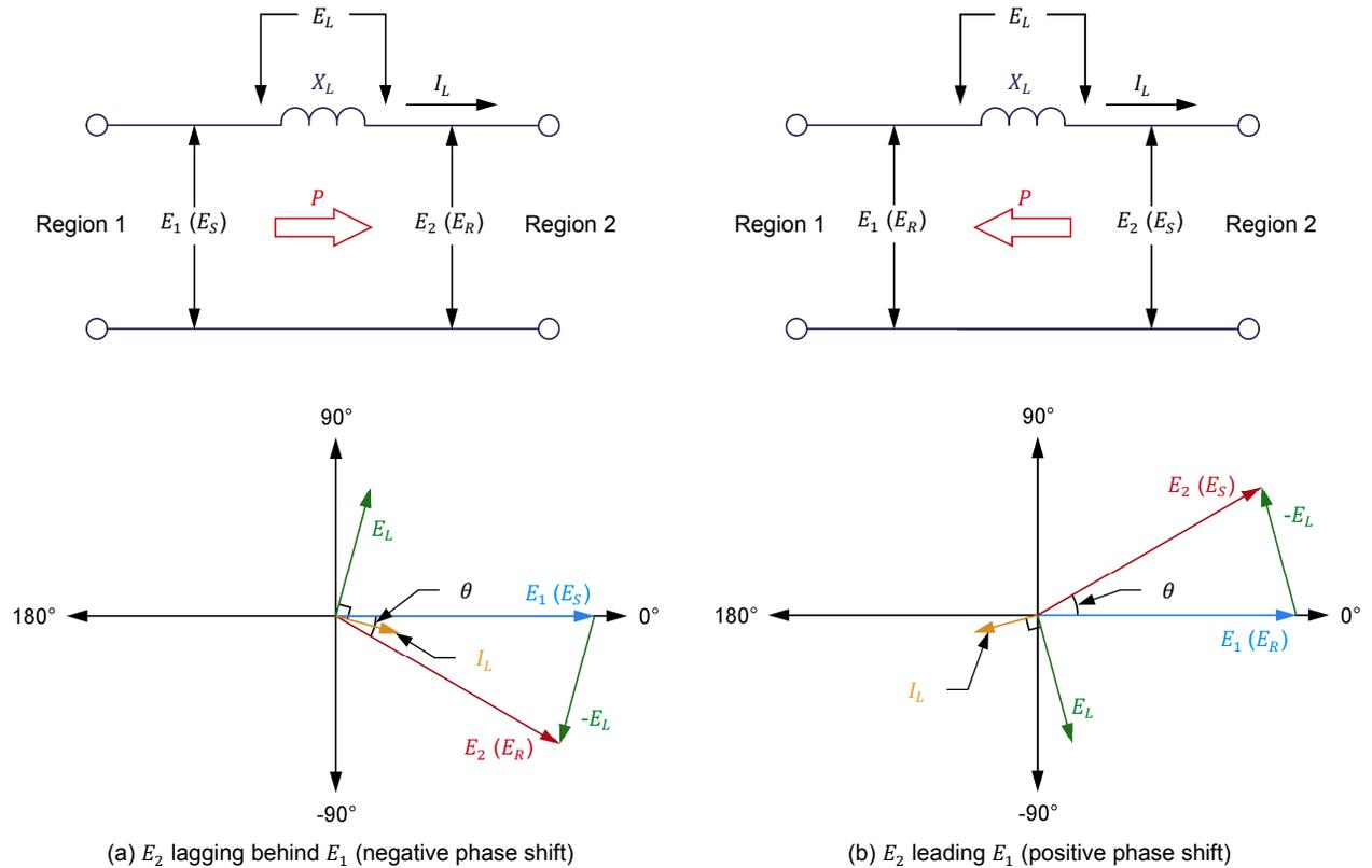
**Figure 29.** The direction of active power flow in an ac transmission line of an interconnected power network depends on the polarity of the phase shift  $\theta$  between the voltages at both ends of the line.
