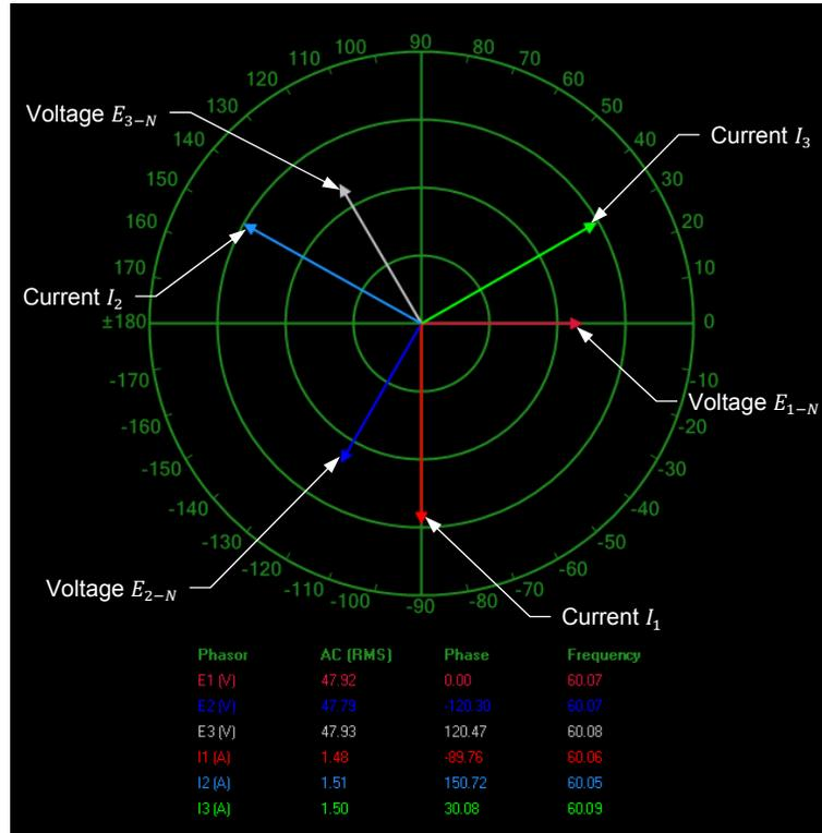
Phasors of the phase voltages  $E_{1-N}$ ,  $E_{2-N}$ , and  $E_{3-N}$  and line currents  $I_1$ ,  $I_2$ , and  $I_3$  at the ac side of the three-phase PWM rectifier/inverter when the reactive current command is equal to -1.5 A and the active current command is set to zero.
