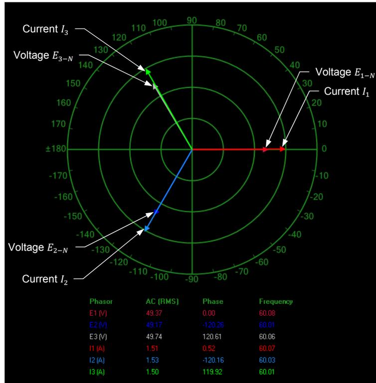
Phasors of the phase voltages  $E_{1-N}$ ,  $E_{2-N}$ , and  $E_{3-N}$  and line currents  $I_1$ ,  $I_2$ , and  $I_3$  at the ac side of the three-phase PWM rectifier/inverter when the active current command is equal to 1.5 A and the reactive current command is set to zero.
