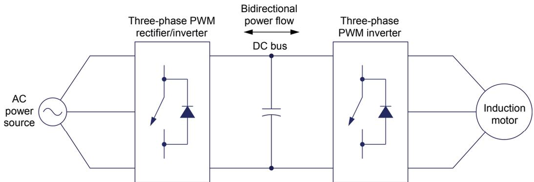
**Figure 14.** Three-phase induction motor drive using a three-phase PWM rectifier/inverter for ac-to-dc power conversion.
