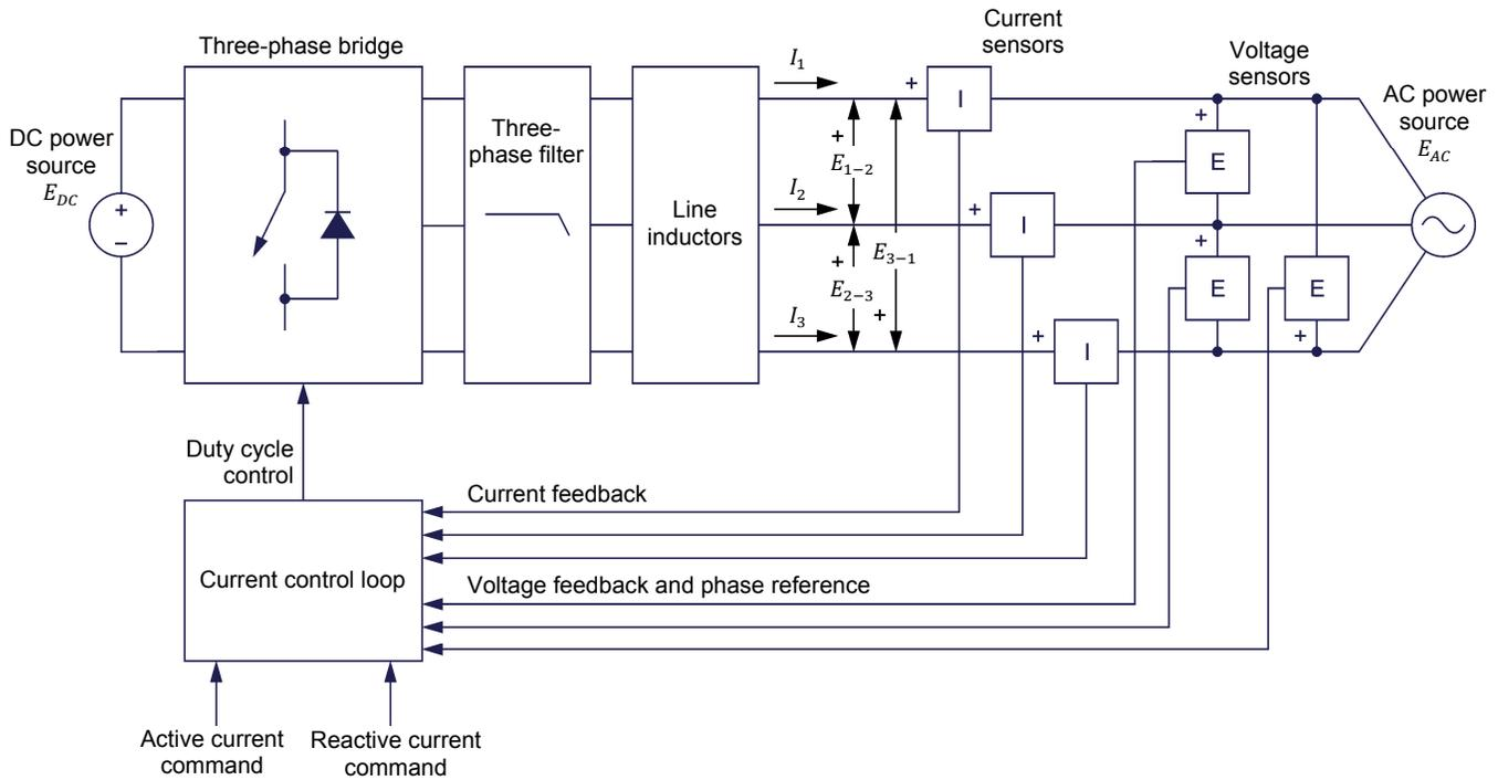
Figure 8. Block diagram of a three-phase PWM rectifier/inverter connected to a dc power source and an ac power source.
