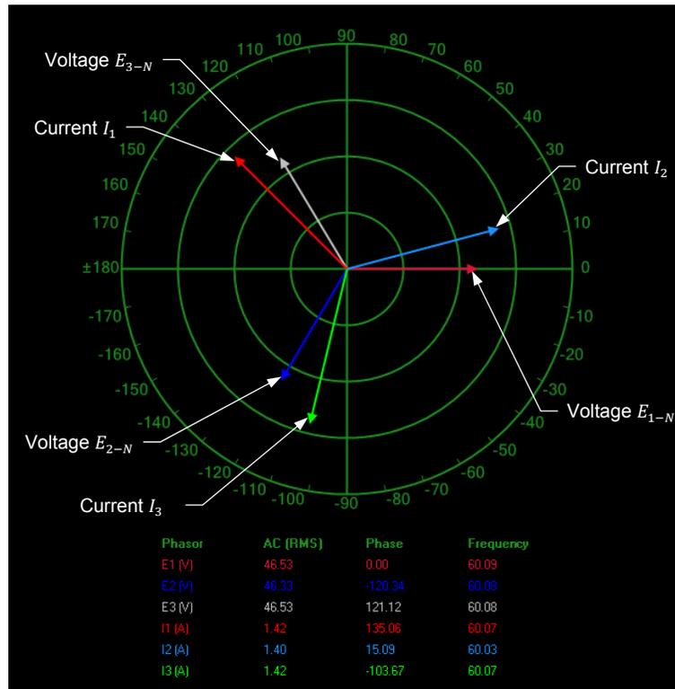
Phasors of the phase voltages  $E_{1-N}$ ,  $E_{2-N}$ , and  $E_{3-N}$  and line currents  $I_1$ ,  $I_2$ , and  $I_3$  at the ac side of the three-phase PWM rectifier/inverter when the active current command is equal to -1.0 A and the reactive current command is equal to 1.0 A.
