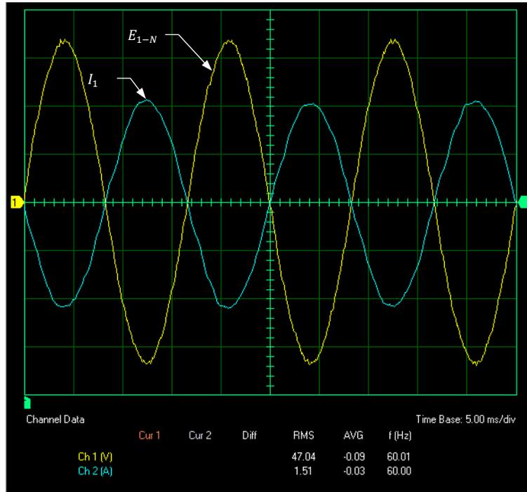
Waveforms of phase voltage  $E_{1-N}$  and line current  $I_1$  at the ac side of the three-phase PWM rectifier/inverter when the active current command is equal to -1.5 A and the reactive current command is set to zero.
