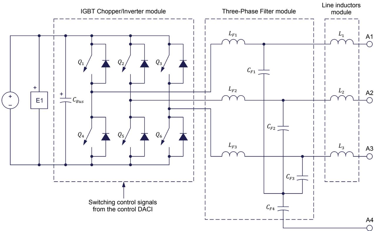
Figure 17. Three-phase PWM rectifier/inverter connected to a dc power source and a three-phase ac power source.
