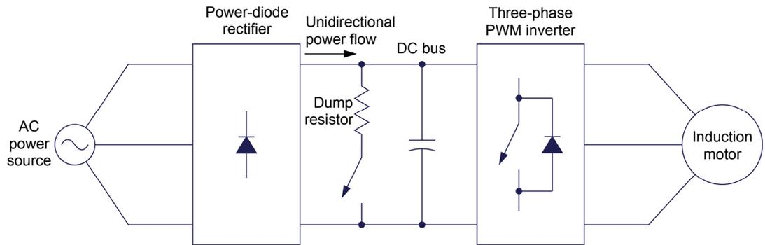
**Figure 13.** Three-phase induction motor drive using a power-diode three-phase rectifier for ac-to-dc power conversion.
