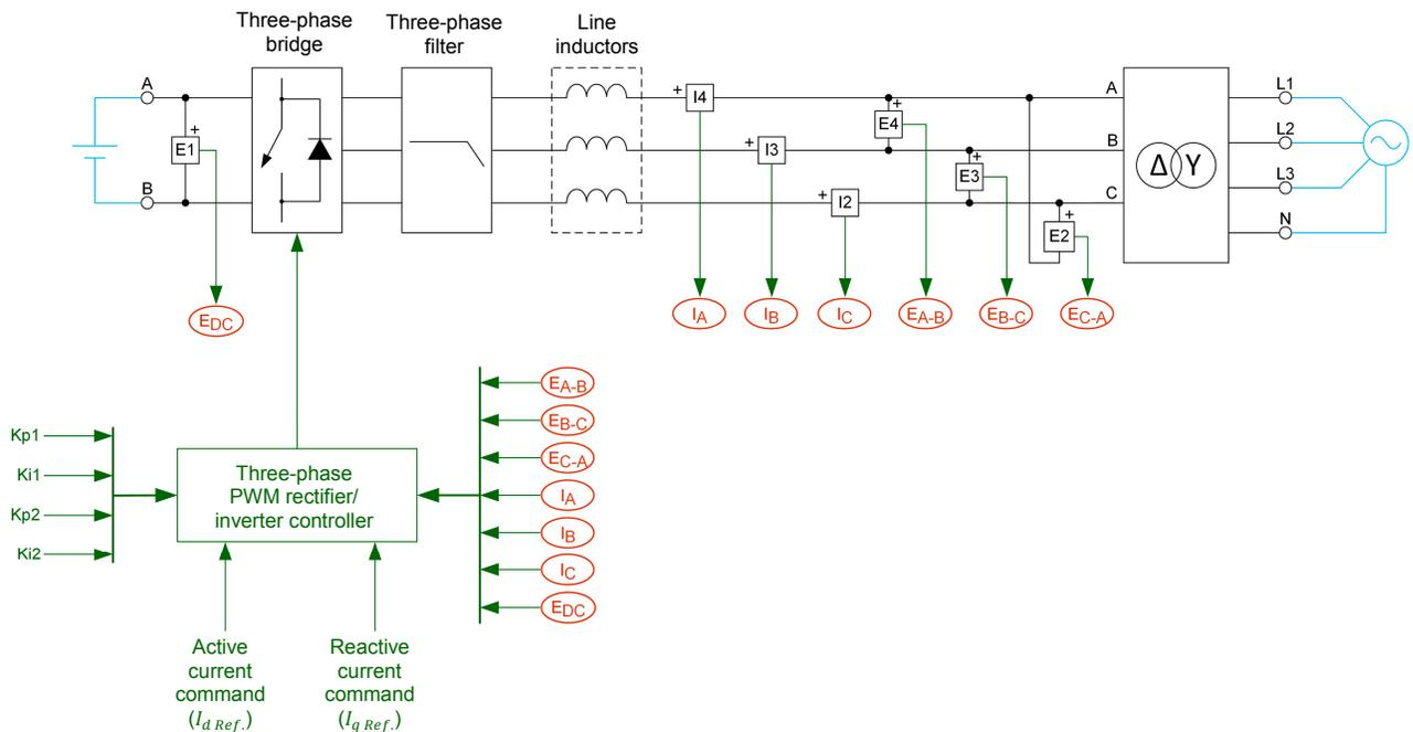
Figure 16. Block diagram of a three-phase PWM rectifier/inverter.
