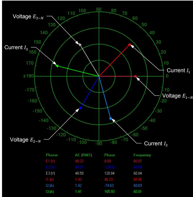
Phasors of the phase voltages  $E_{1-N}$ ,  $E_{2-N}$ , and  $E_{3-N}$  and line currents  $I_1$ ,  $I_2$ , and  $I_3$  at the ac side of the three-phase PWM rectifier/inverter when the active current command and the reactive current command are both equal to 1.0 A.
