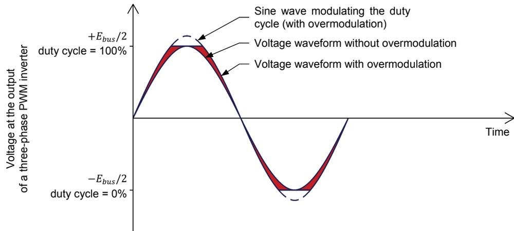
Figure 9. Voltage waveform at the output of a PWM inverter with and without overmodulation (after filtering).
