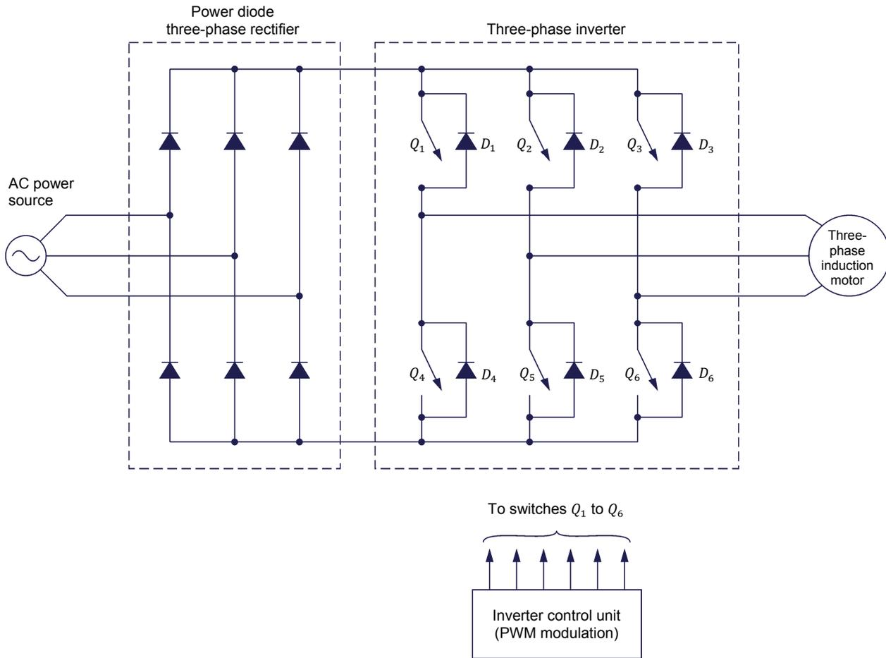
Figure 3. Simplified diagram of a three-phase induction-motor drive.
