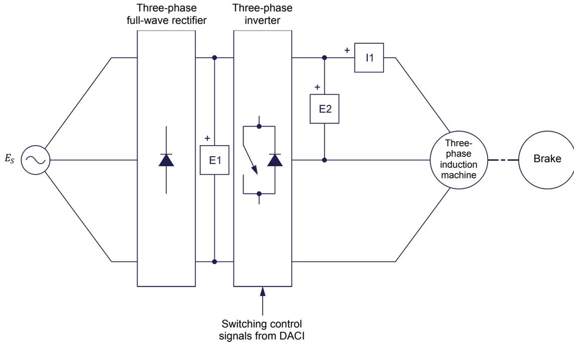
Figure 11. Three-phase, variable-frequency induction-motor drive (without three-phase filter).
