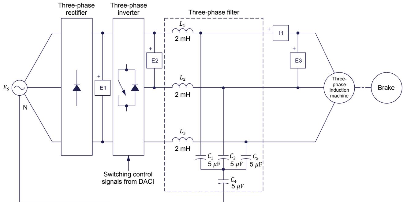
Figure 10. Three-phase, variable-frequency induction-motor drive (with three-phase filter).
