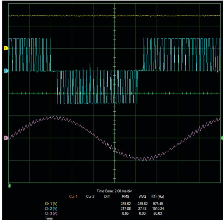
Voltage and current waveforms obtained when the three-phase, variable-frequency drive operates at motor nominal frequency (without overmodulation).
