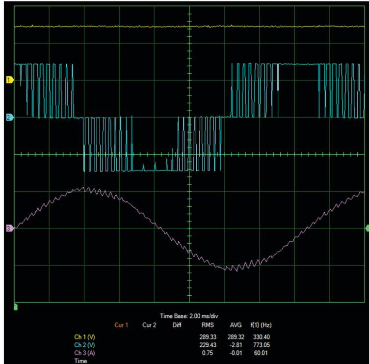
Voltage and current waveforms obtained when the three-phase, variable-frequency drive operates at motor nominal frequency (with overmodulation).
