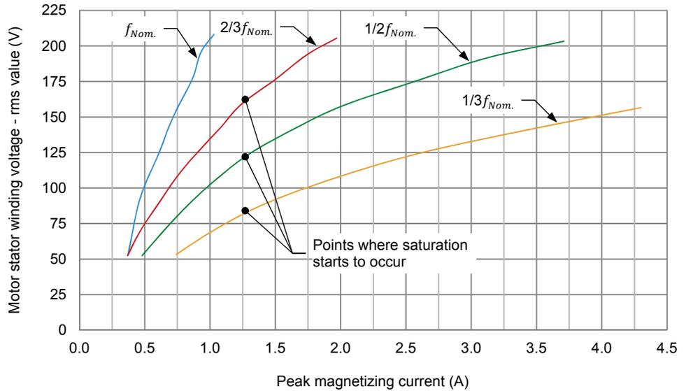
Saturation curves of the three-phase induction motor at various operating frequencies.
