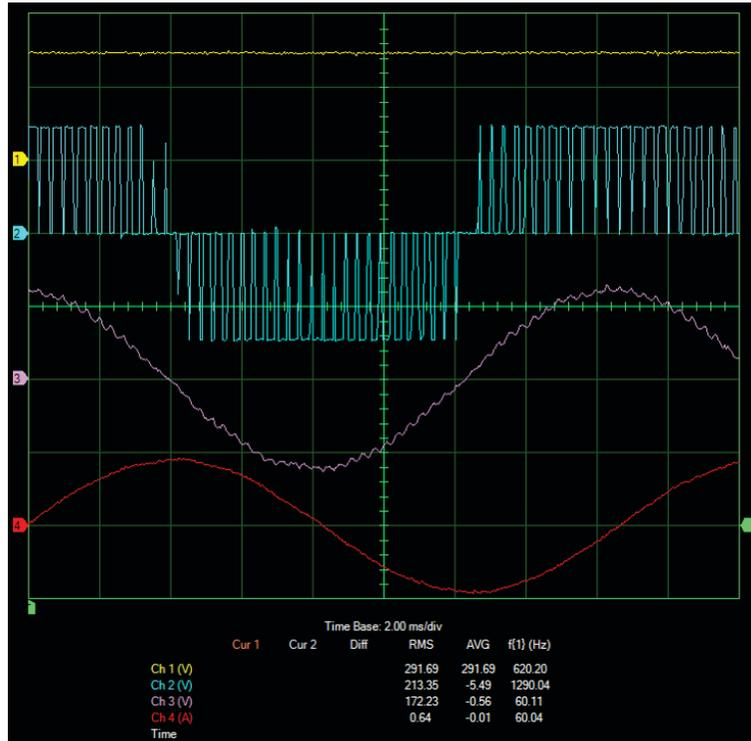
Voltage and current waveforms obtained when the three-phase, variable-frequency induction-motor drive operates at motor nominal frequency.
