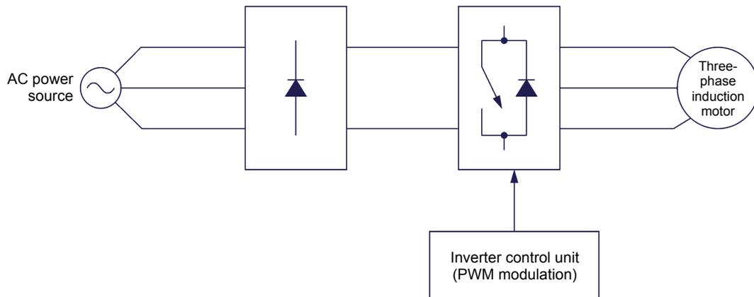
Figure 4. Simplified diagram of a three-phase induction-motor drive using symbols that represent a power diode three-phase rectifier and a three-phase inverter.
