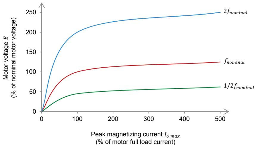
Figure 7. Typical saturation curves of an induction motor at various frequencies (motor voltage as a function of the magnetizing current).
