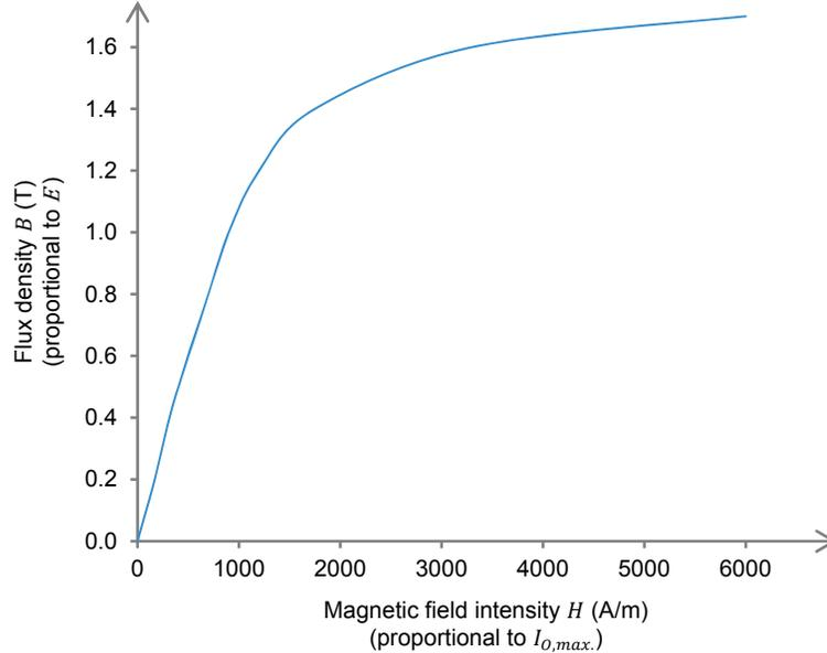
**Figure 5. Typical saturation curve of an induction motor (flux density  $B$  as a function of the magnetic field intensity  $H$ ).**
