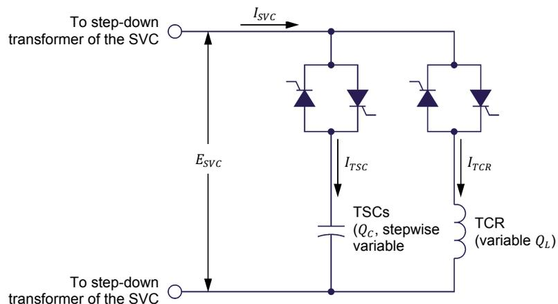
Figure 35. Simplified circuit diagram of one leg (phase) of an SVC of the TCR-TSC type showing the main voltage, current, and reactive power parameters.
