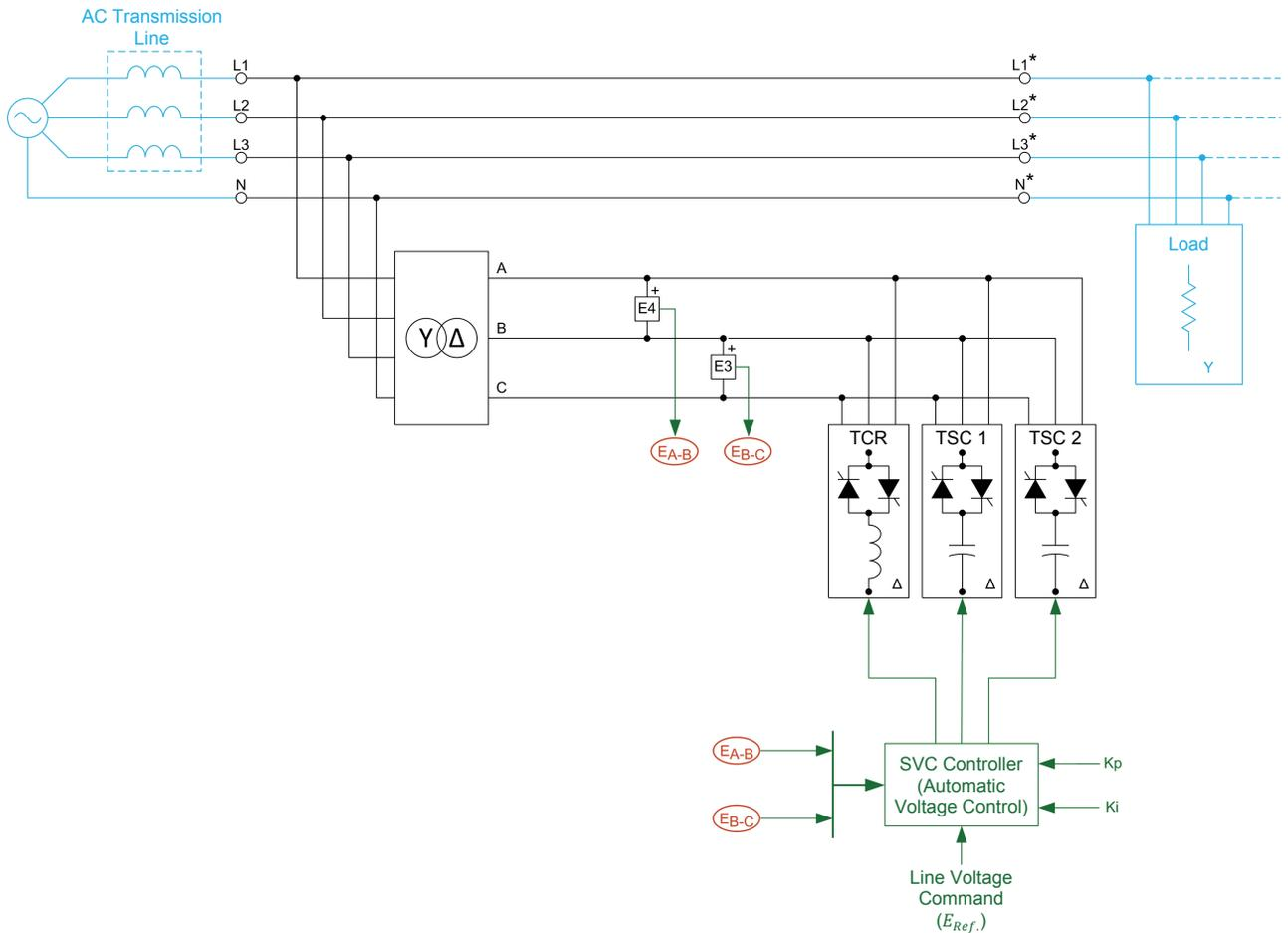
Figure 38. Block diagram of an SVC designed for voltage compensation.
