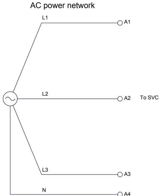
**Figure 40.** Circuit for measuring the reactive power capacity of an SVC consisting of one TCR and two TSCs.
