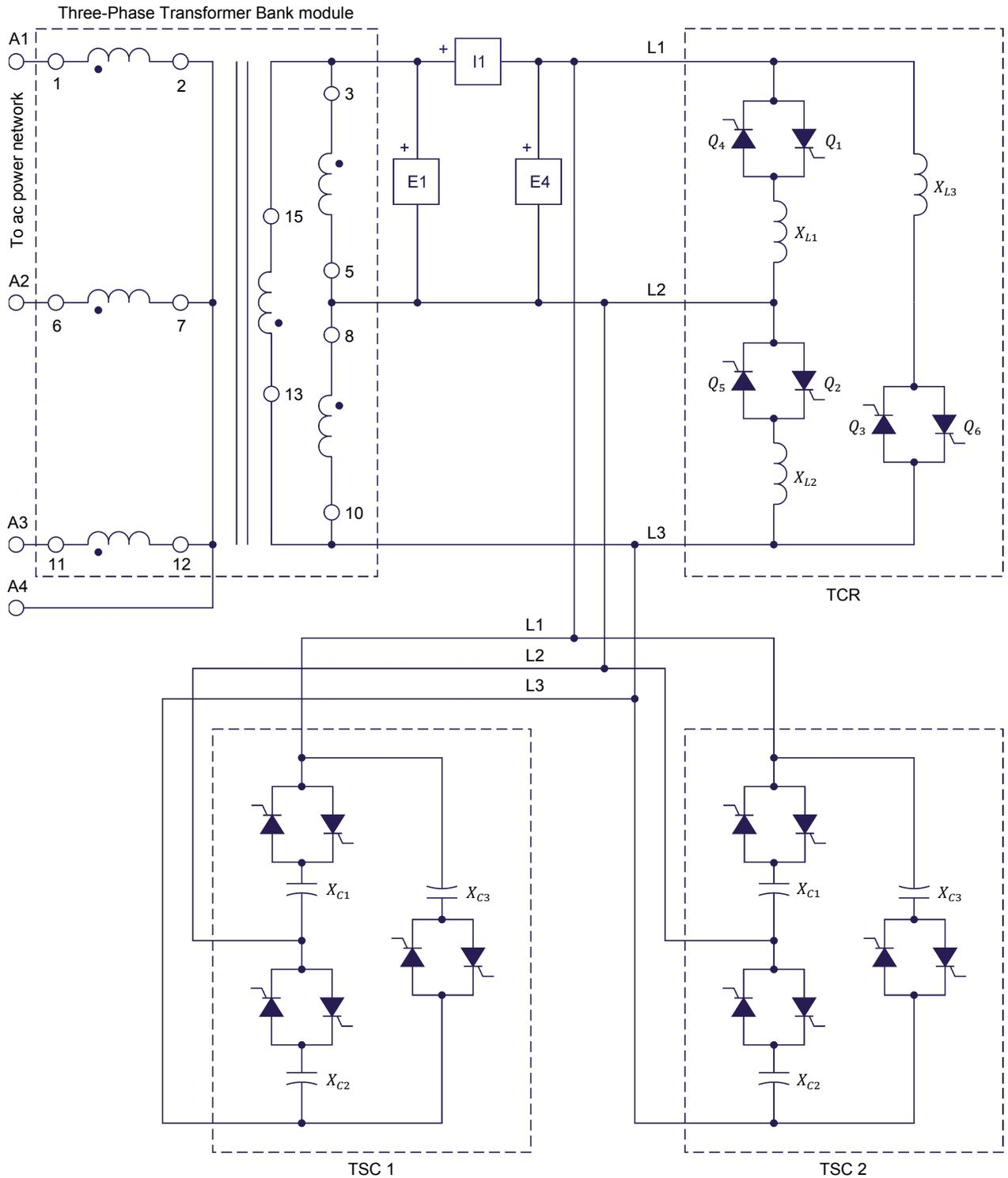
Figure 41. Circuit for measuring the reactive power capacity of an SVC consisting of one TCR and two TSCs.
