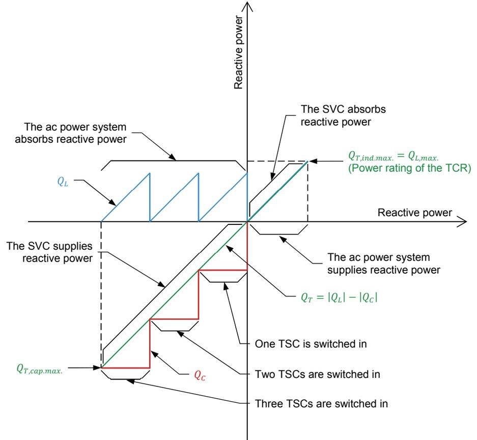
Figure 36. Reactive power exchange characteristic of an SVC of the TCR-TSC-type.
