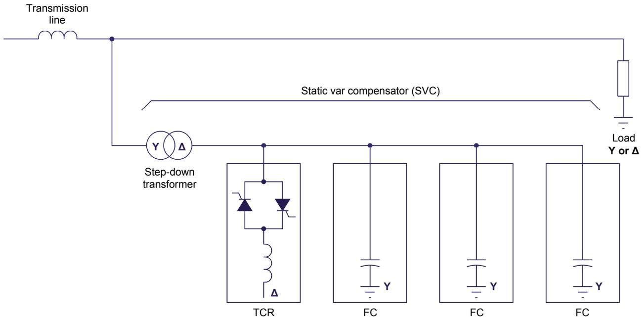
Figure 31. Simplified single-wire circuit diagram of an SVC of the TCR-FC type.
