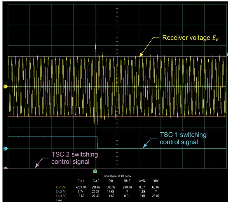
Receiver voltage  $E_R$ , TSC 1 switching control signal, and TSC 2 switching control signal when the SVC compensates the voltage at the receiver end of a long ac transmission line and the load decreases.
