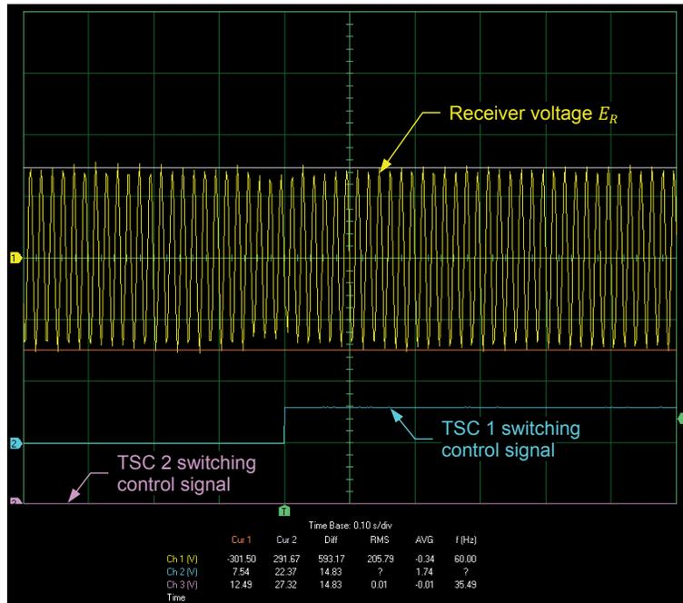
Receiver voltage  $E_R$ , TSC 1 switching control signal, and TSC 2 switching control signal when the SVC compensates the voltage at the receiver end of a long ac transmission line and the voltage compensation provided by the shunt-capacitor substation decreases.
