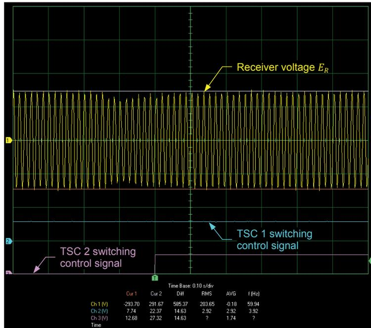
Receiver voltage  $E_R$ , TSC 1 switching control signal, and TSC 2 switching control signal when the SVC compensates the voltage at the receiver end of an ac transmission line and the load increases.
