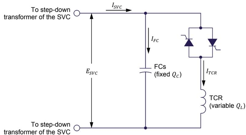
Figure 32. Simplified circuit diagram of one leg (phase) of an SVC of the TCR-FC-type showing the main voltage, current, and reactive power parameters.
