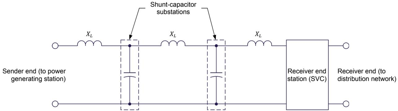
**Figure 29. Typical ac transmission line used to transfer large amounts of electrical power over a long distance from a power generating station to the distribution network.**
