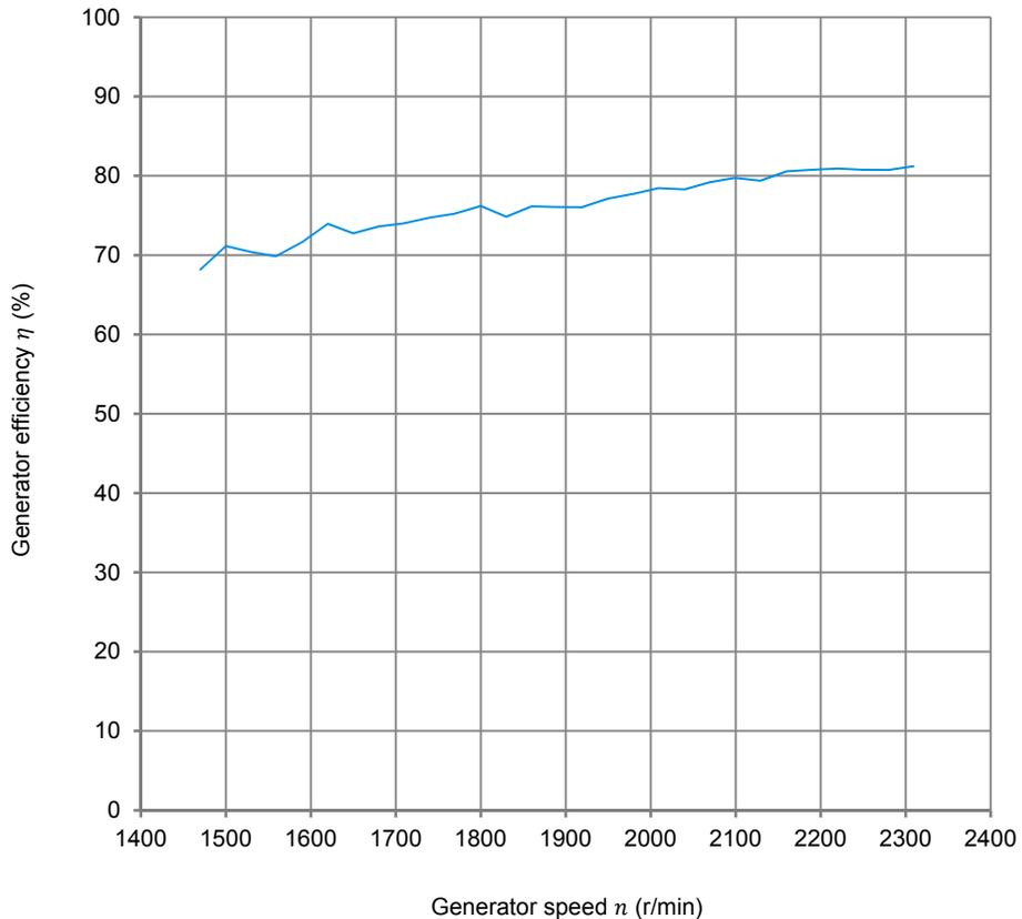
Doubly-fed induction generator efficiency  $\eta$  as a function of the generator synchronous speed  $n_s$ .
