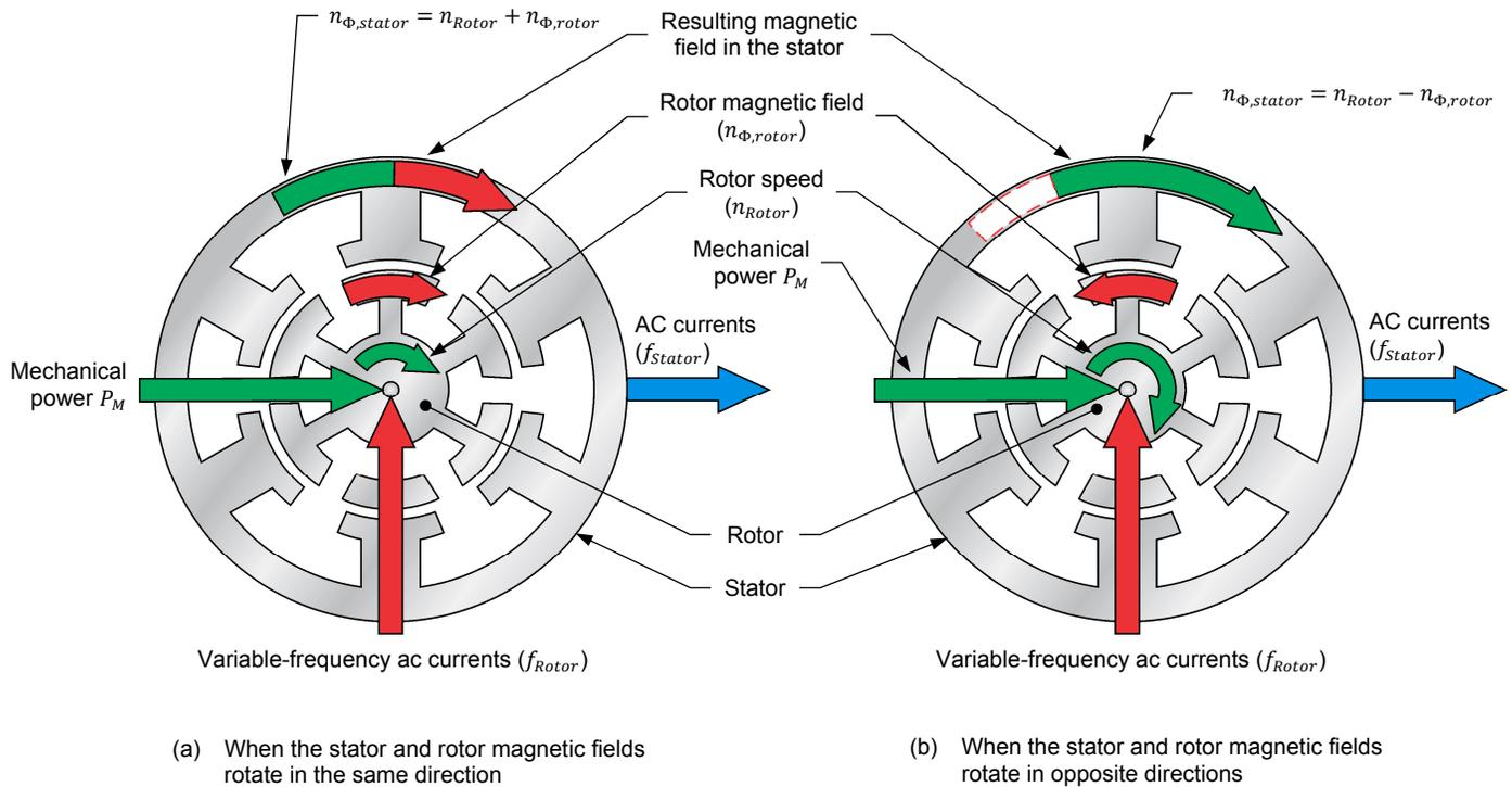
**Figure 10.** Interaction between the rotor speed and the frequency of the rotating magnetic field created in the rotor windings of a doubly-fed induction generator.
