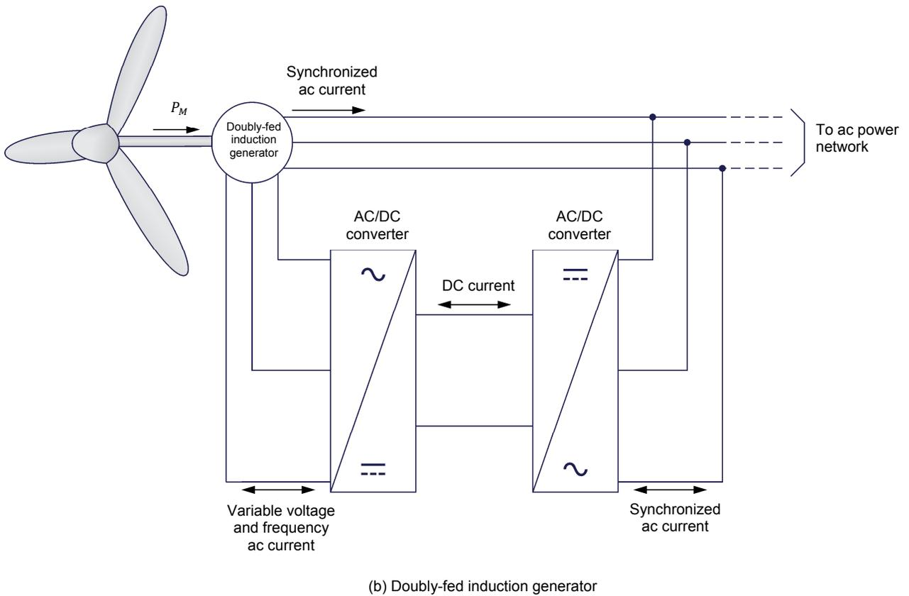
Figure 11. Circuit topologies for two types of generators found in variable-speed wind turbines.
