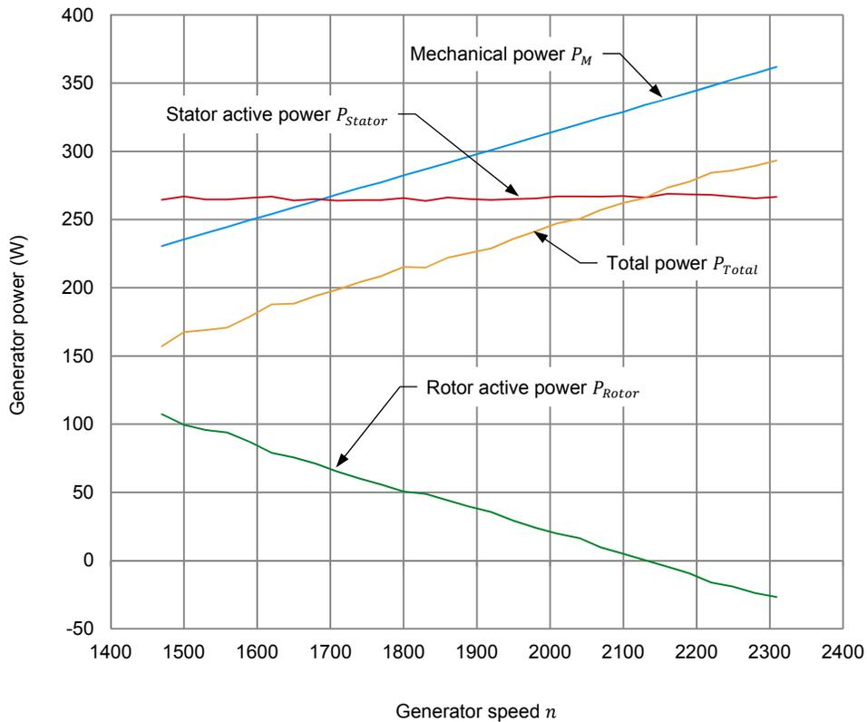
Doubly-fed induction generator mechanical power  $P_M$ , active power at the stator  $P_{Stator}$ , active power at the rotor  $P_{Rotor}$ , and total power  $P_{Total}$  as a function of the generator speed  $n$ .
