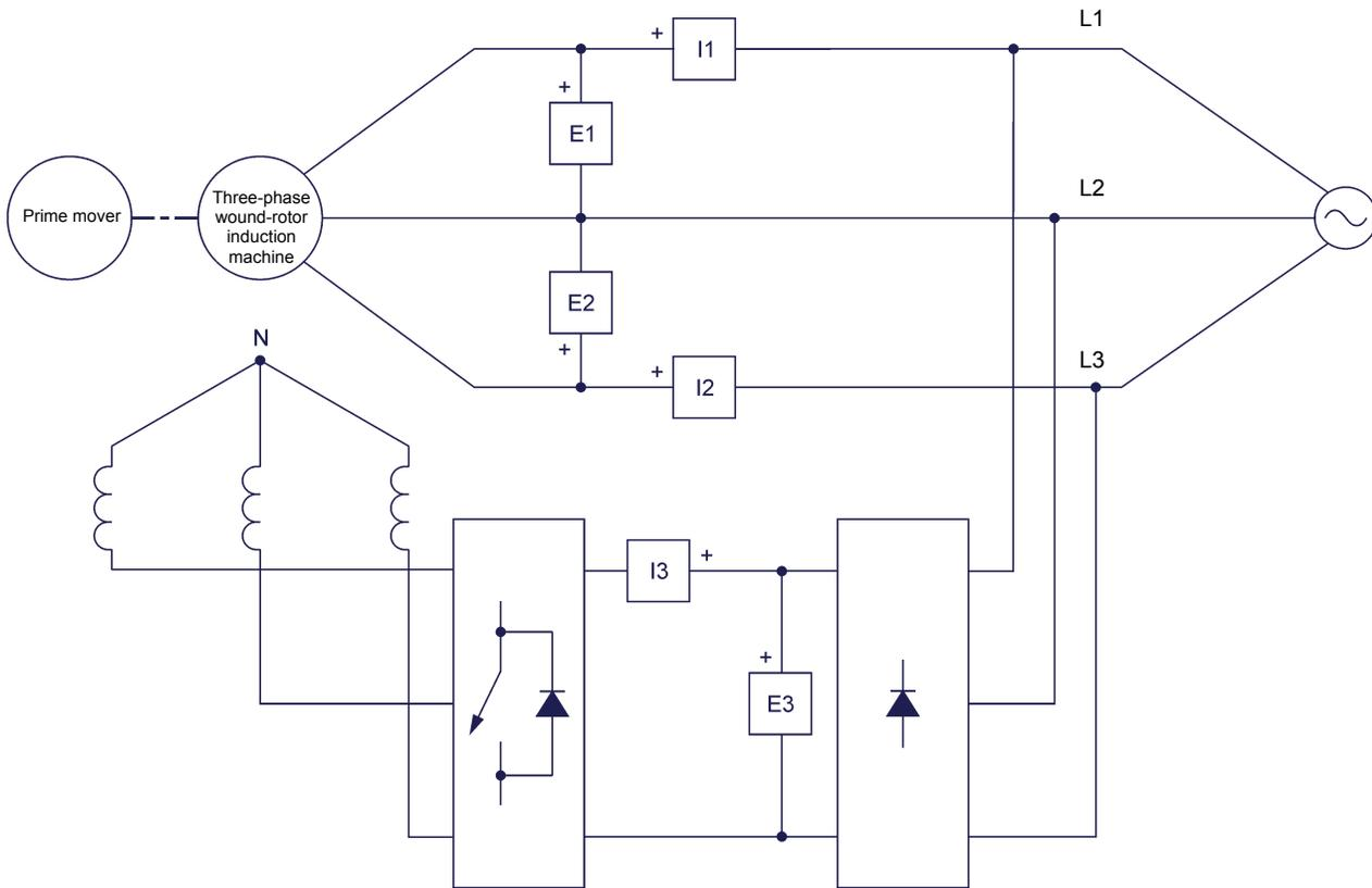
**Figure 12.** Three-phase wound-rotor induction machine operating as a doubly-fed induction generator.
