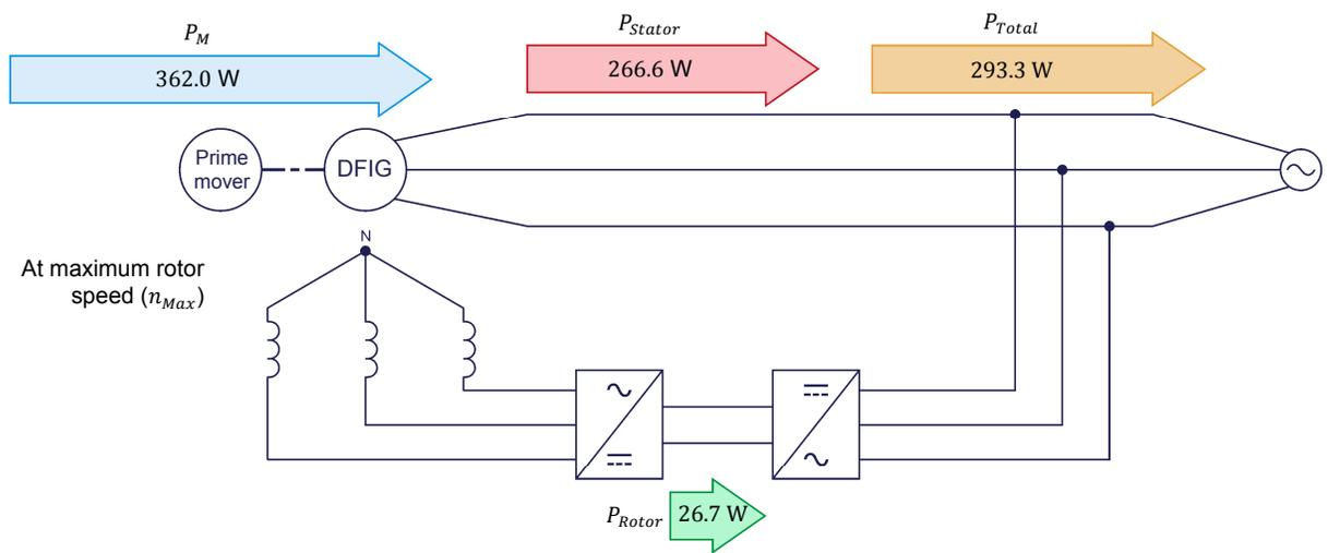
Power balance of the doubly-fed induction generator when the generator rotates at minimum speed, singly-fed synchronous speed, and maximum speed.
