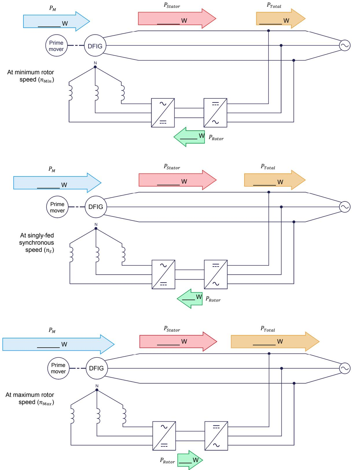
Figure 13. Power balance of the doubly-fed induction generator when the generator rotates at minimum speed, singly-fed synchronous speed, and maximum speed.
