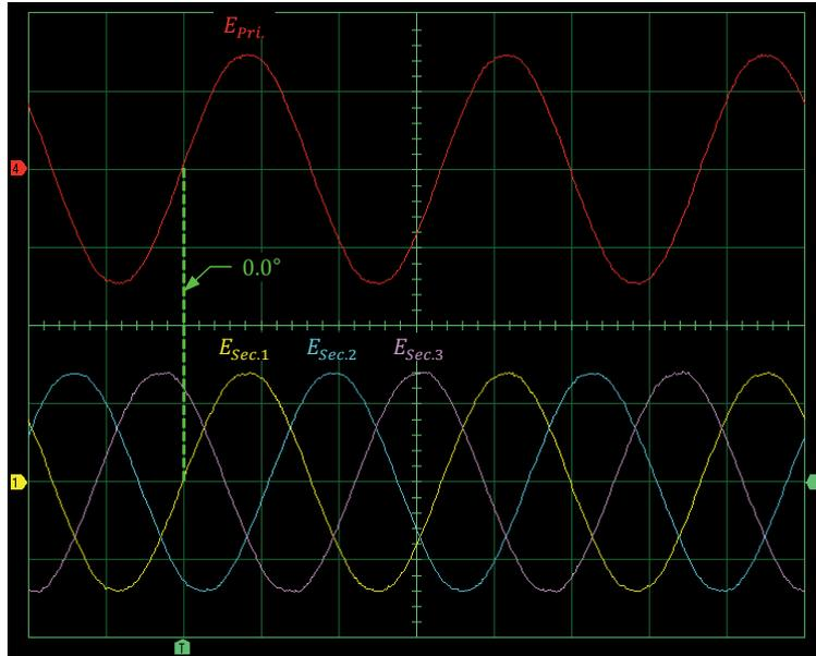
Sine waves of the line voltages at the primary and the secondary of the three-phase transformer bank when it is connected in a wye-wye configuration.
