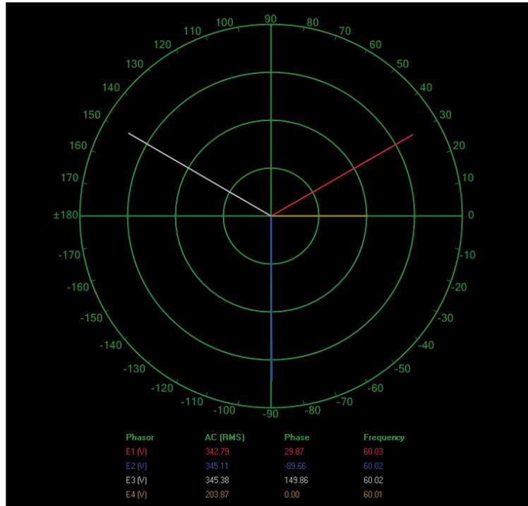
Phasors of the line voltages at the primary and the secondary of the three-phase transformer bank when it is connected in a delta-ye configuration.
