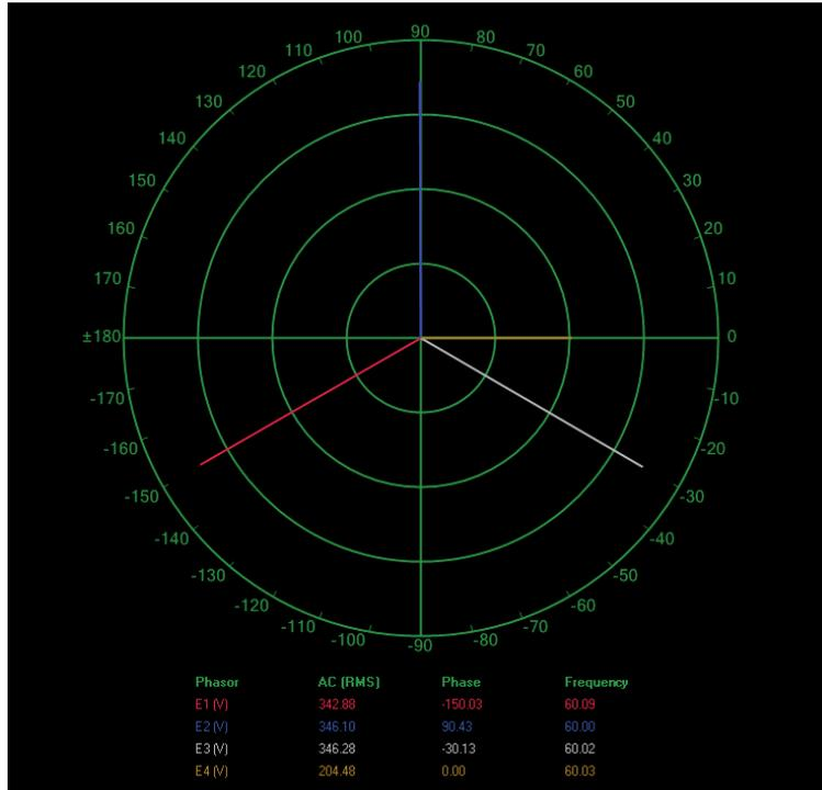
Phasors of the line voltages at the primary and the secondary of the three-phase transformer bank when it is connected in a delta-wye configuration with reversed connections at the secondary windings.
