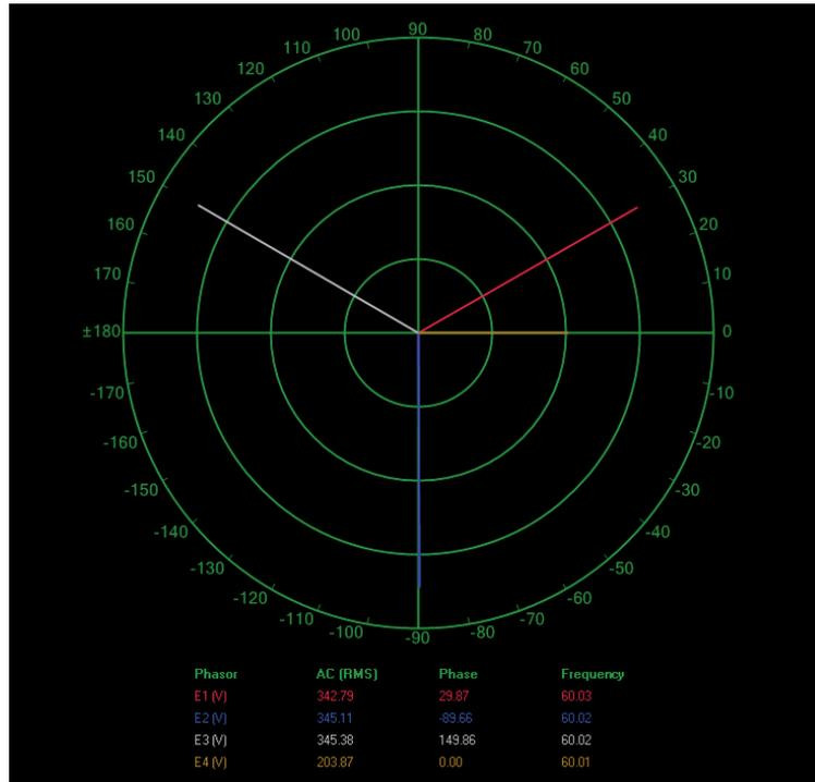
Phasors of the line voltages at the primary and the secondary of the three-phase transformer bank when it is connected in a delta-*wye* configuration.
