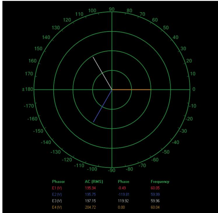
Phasors of the line voltages at the primary and the secondary of the three-phase transformer bank when it is connected in a wye-wye configuration.
