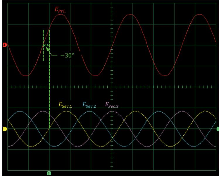
Sine waves of the line voltages at the primary and the secondary of the three-phase transformer bank when it is connected in a wye-delta configuration.
