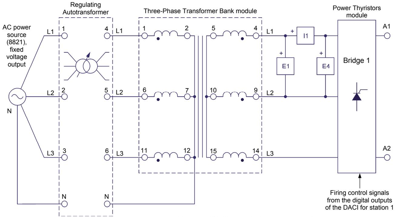
Figure 50. HVDC transmission system (part I).
