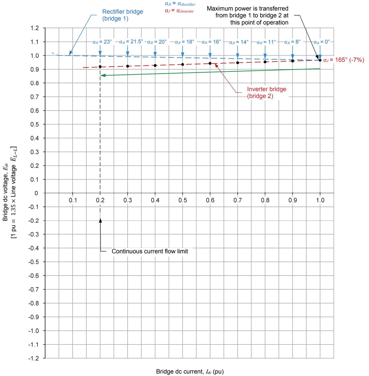
Figure 47. The amount of power transferred through an HVDC transmission system is set by adjusting the dc line current, i.e., the current command  $I_{Ref. (rectifier)}$ . To keep power losses ( $RI^2$  losses) to a minimum and to ensure a good DPF at both thyristor bridges, the system is set to operate at the highest dc voltage possible.
