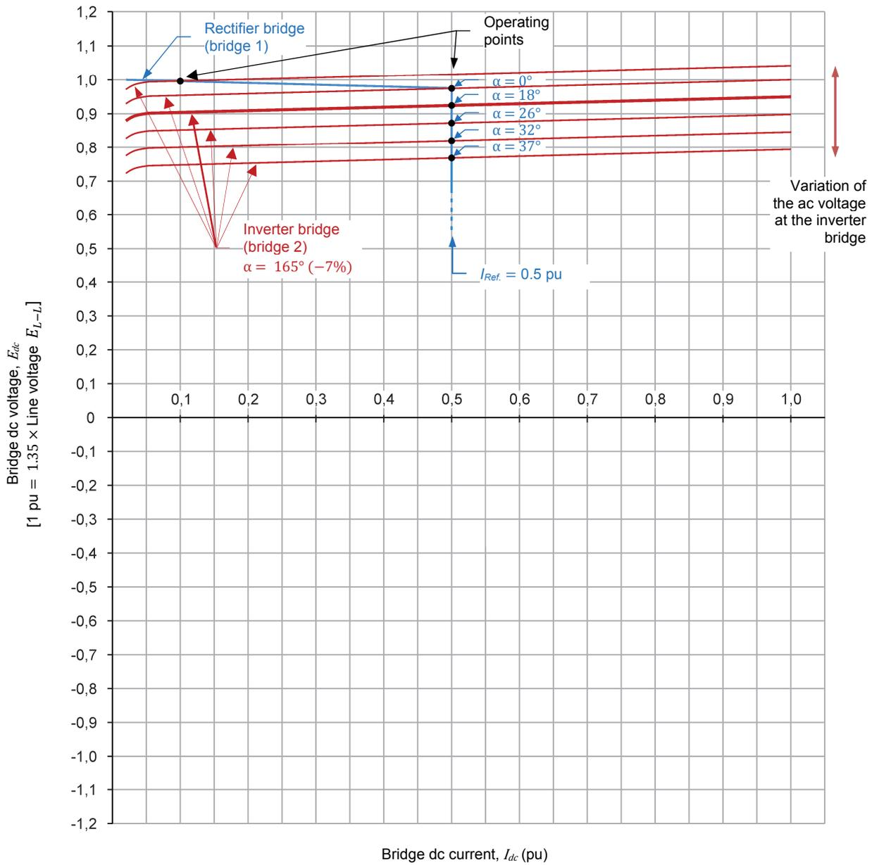
Figure 38. When ac voltage fluctuations occur at the inverter bridge, the current control loop at the rectifier bridge readjusts the firing angle of the rectifier bridge to keep the dc line current  $I_{dc}$  at the value of the current command  $I_{Ref.}$  (0.5 pu).
