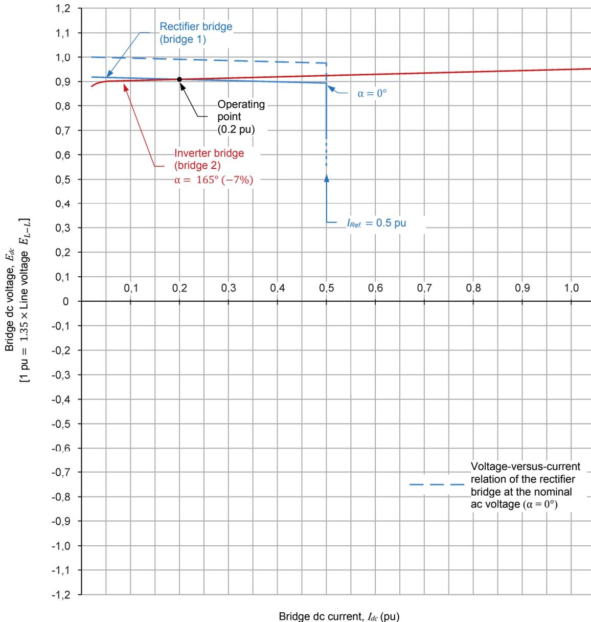
Figure 43. When the ac voltage decreases too much at the rectifier bridge, the current control loop decreases the firing angle of the rectifier bridge to the minimum value ( $0^\circ$ ); this is not sufficient to keep current  $I_{dc}$  at the value of the current command  $I_{Ref}$  (0.5 pu). As a result, current  $I_{dc}$  decreases and becomes lower (0.2 pu in this example) than the current command.
