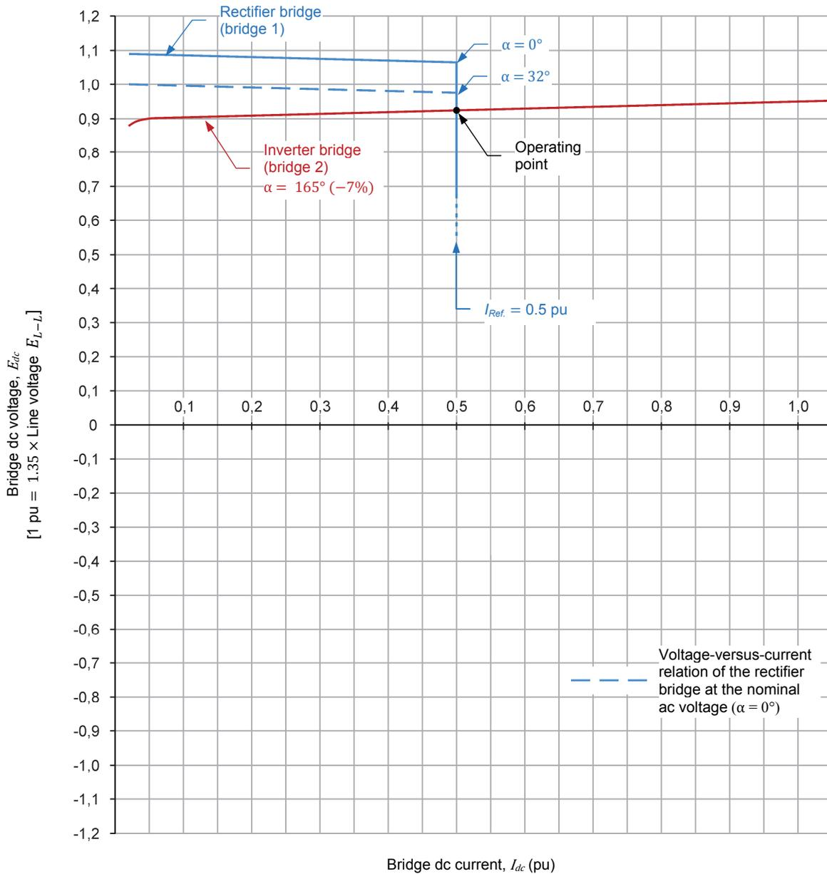
Figure 41. A further increase in the ac voltage at the rectifier bridge causes the current control loop to further increase the firing angle of the rectifier bridge to keep current  $I_{dc}$  at the value of the current command  $I_{Ref.}$  (0.5 pu).
