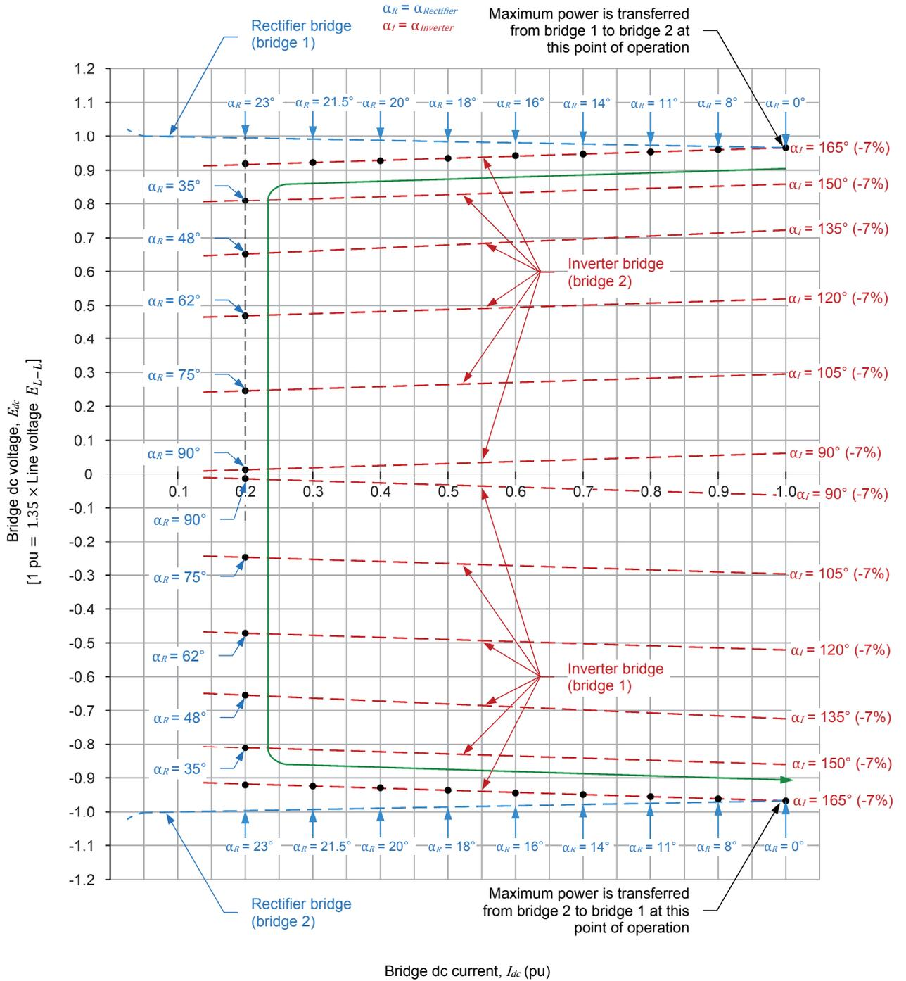
Figure 49. Diagram showing how the direction of power flow is reversed in an HVDC transmission system.
