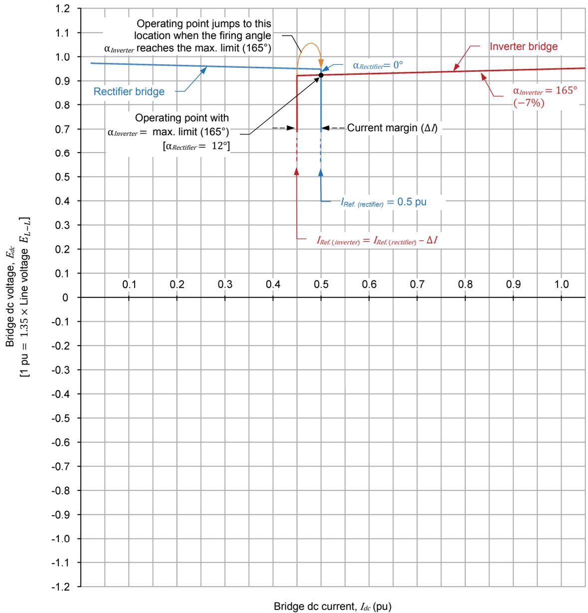
Figure 46. When the ac voltage increases at the rectifier bridge or decreases at the inverter bridge to the extent that the firing angle  $\alpha_{Inverter}$  reaches the maximum value ( $165^\circ$  in our example) and the current  $I_{dc}$  starts increasing significantly, the current control loop of the rectifier bridge enters into action to maintain current  $I_{dc}$  to  $I_{Ref. (rectifier)}$  (i.e., 0.5 pu in the above example).
