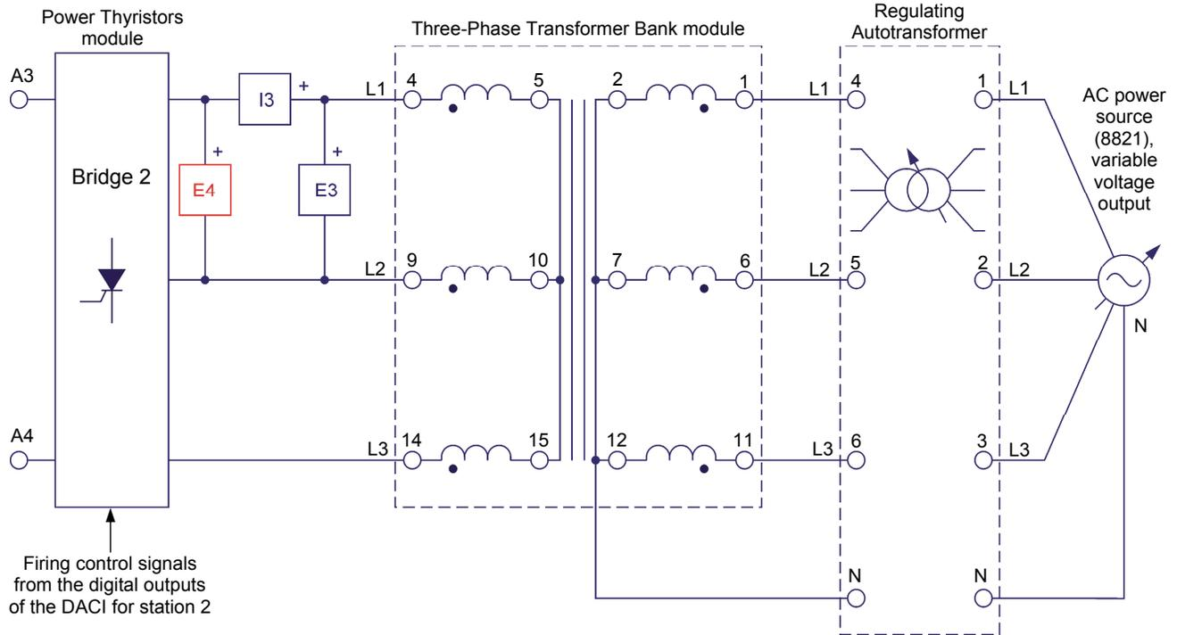
Figure 52. HVDC transmission system (part III).
