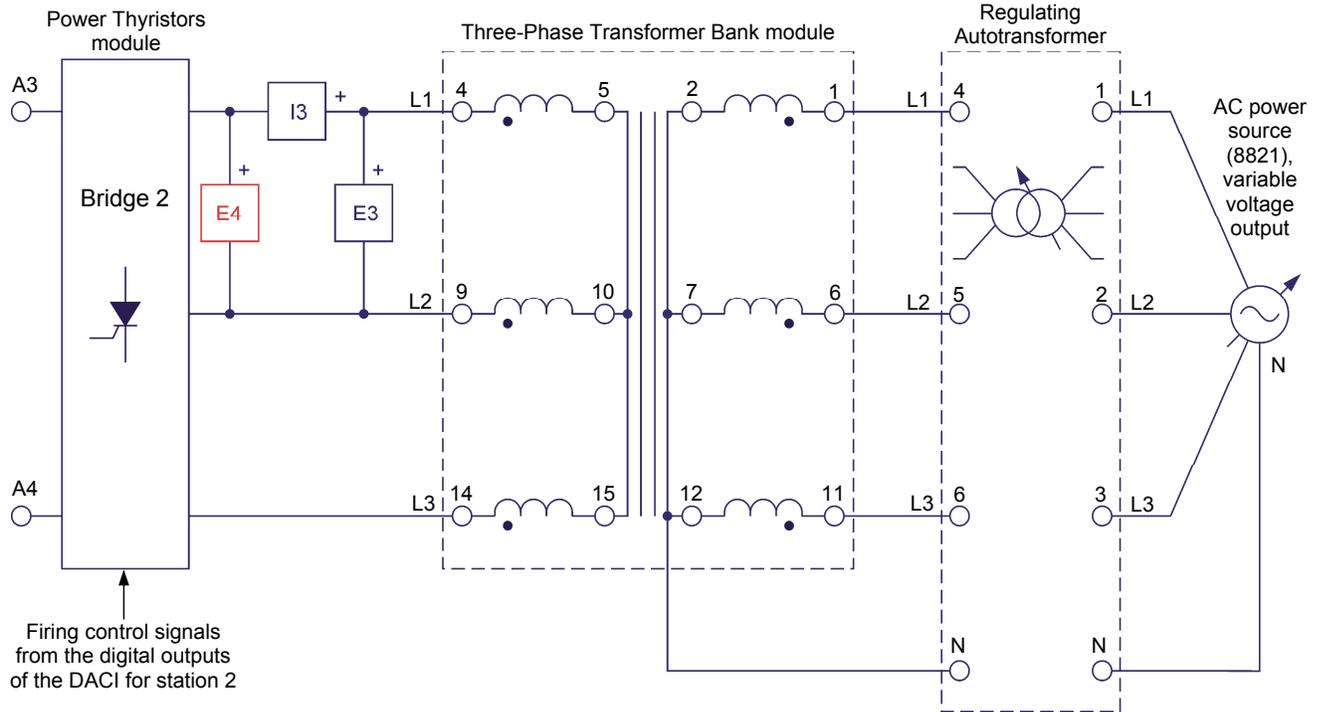
Figure 52. HVDC transmission system (part III).
