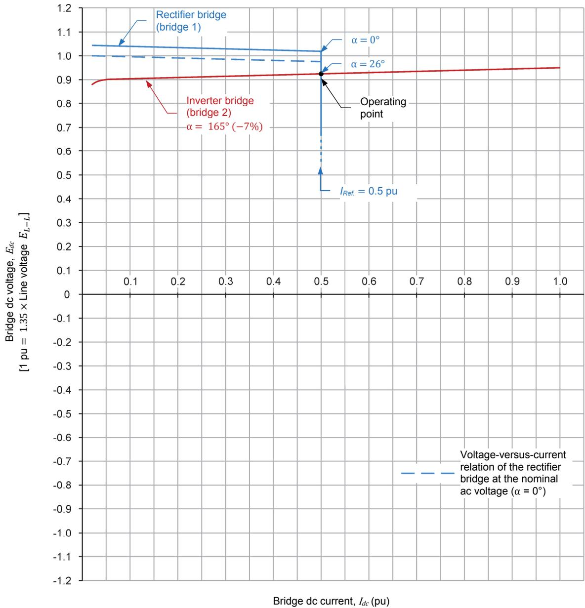
Figure 40. When the ac voltage increases at the rectifier bridge, the current control loop increases the firing angle of the rectifier bridge to keep the dc line current  $I_{dc}$  at the value of the current command  $I_{Ref}$  (0.5 pu).
