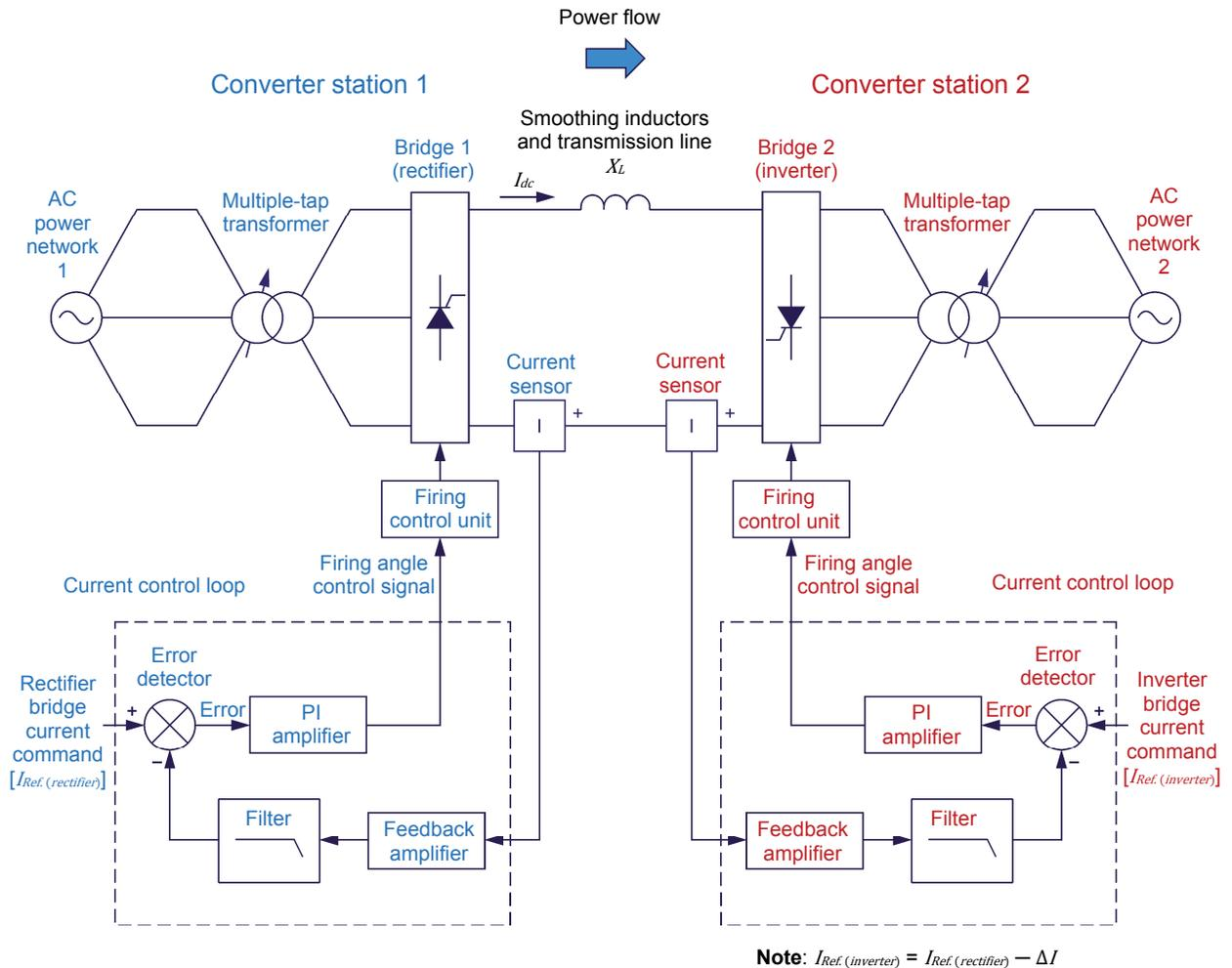
Figure 44. The addition of a second current control loop at the inverter bridge of an HVDC transmission system limits the effect of ac voltage fluctuations on the dc line current  $I_{dc}$  by keeping it within a predetermined current margin ( $\Delta I$ ).
