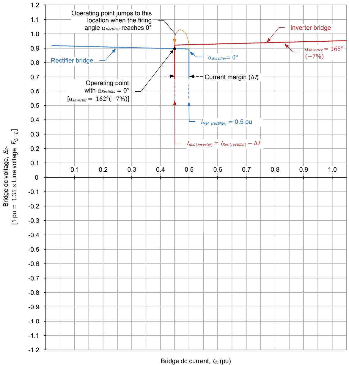
Figure 45. When the ac voltage decreases at the rectifier bridge or increases at the inverter bridge to the extent that the firing angle  $\alpha_{Rectifier}$  reaches the minimum value ( $0^\circ$ ) and the current  $I_{dc}$  starts decreasing significantly, the current control loop of the inverter bridge enters into action to maintain current  $I_{dc}$  to  $I_{Ref. (rectifier)} - \Delta I$  (i.e., 0.45 pu in the above example).
