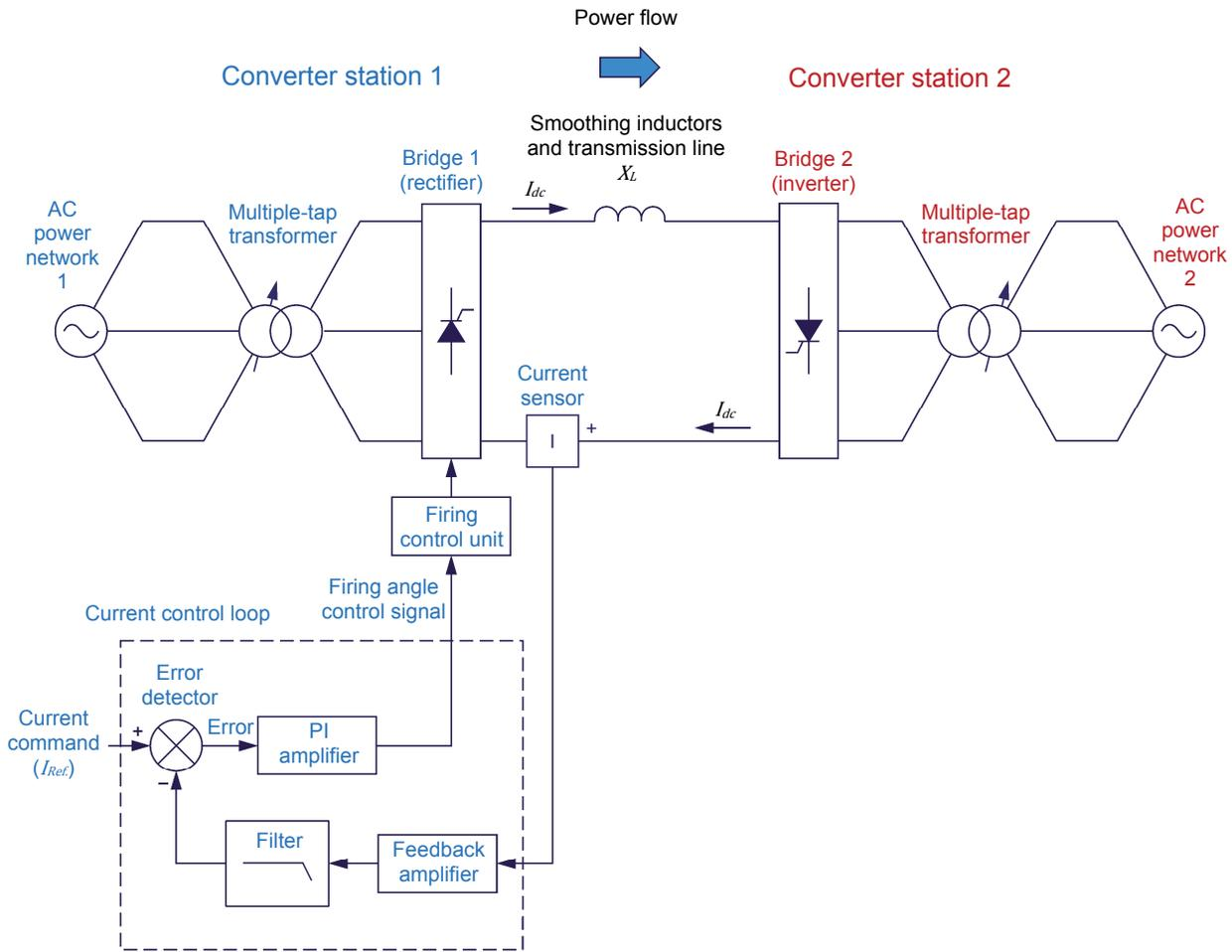
Figure 36. Current control loop used at the rectifier bridge of an HVDC transmission system.
