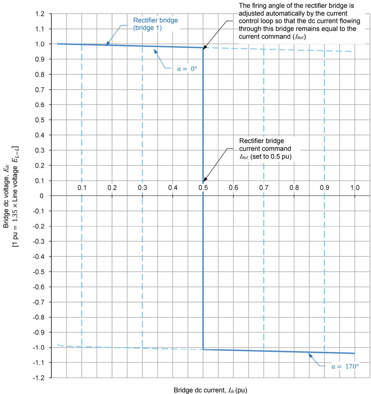
Figure 37. Voltage-versus-current relation at the dc side of the rectifier bridge.
