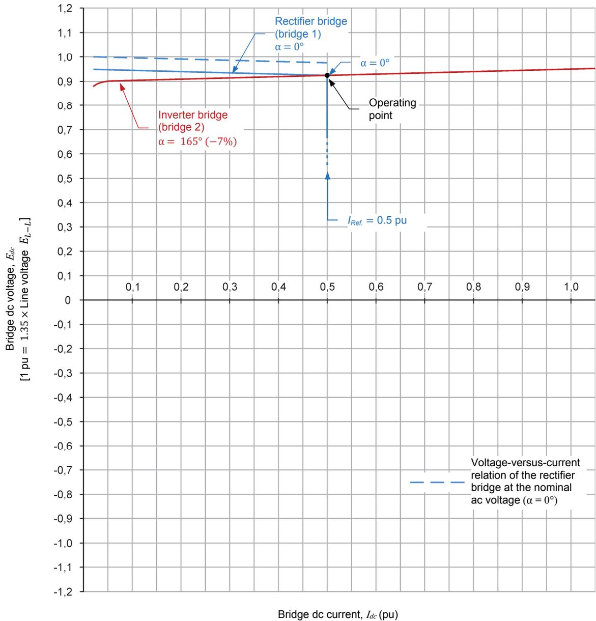
Figure 42. When the ac voltage decreases at the rectifier bridge, the current control loop decreases the firing angle of the rectifier bridge to keep current  $I_{dc}$  at the value of the current command  $I_{Ref}$  (0.5 pu).
