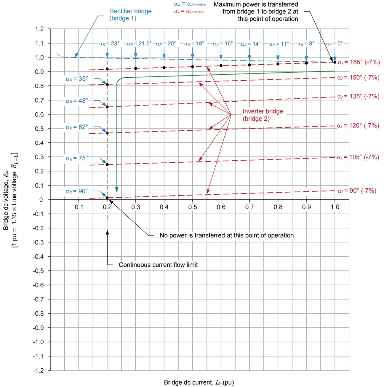
Figure 48. To decrease the amount of power transferred through an HVDC transmission system to zero, the dc voltage at which the system operates is reduced to zero. This, however, results in poor DPFs at both the rectifier and inverter bridges.
