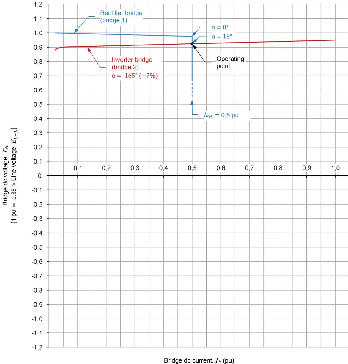
**Figure 39. Voltage-versus-current relations of the rectifier and inverter bridges at the nominal ac voltage.**
